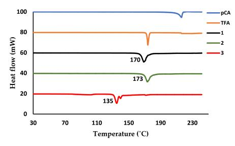
**Figure 9.** Differential scanning calorimetry (DSC) plot of *p*CA (blue), TFA (brown), salt **1** (black), salt **2** (green) and salt **3** (red).
