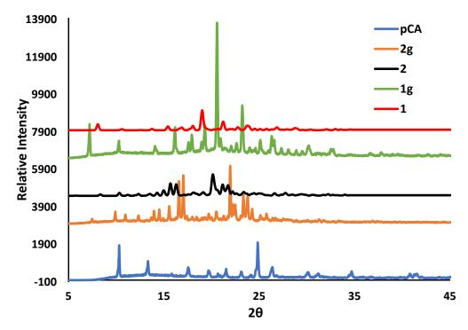
**Figure 6.** PXRD patterns for *p*CA, the ground products **1g** and **2g** after 30 min and the calculated organic salts **1** and **2**.
