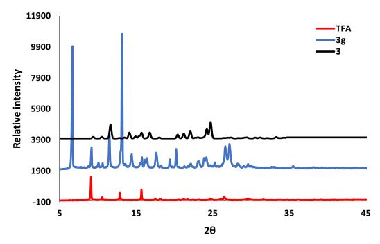
**Figure 7.** PXRD pattern for TFA compared with the ground product **3g** after 20 min and the calculated organic salt **3**.
