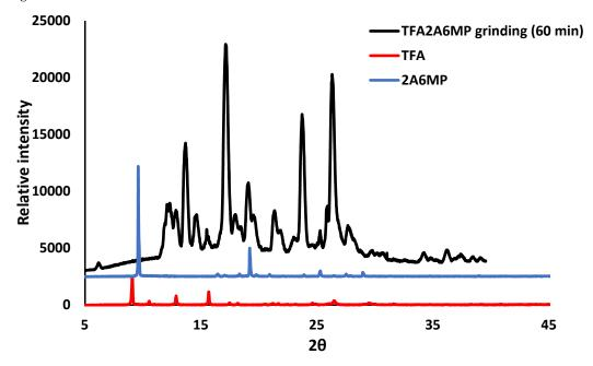
**Figure 8.** PXRD analyses of the ground product of TFA and 2A6MP after 60 min (black), TFA (red) and 2A6MP (blue).
