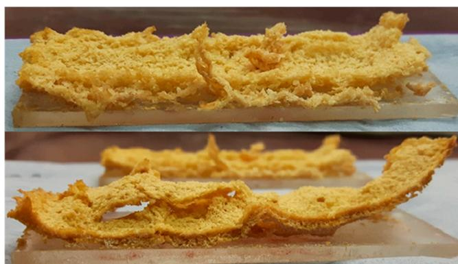
**Figure 11.** Coatings of PVPA/10% chitosan (top) and PVPA/20% chitosan (bottom) applied to PMMA after water soak testing.
