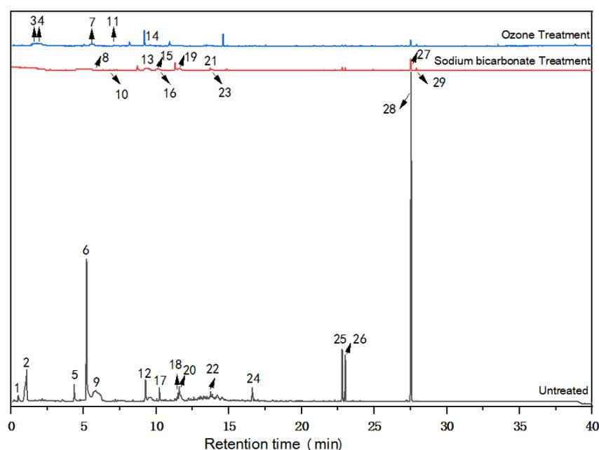
**Figure 2.** Gas chromatography-mass spectrometry (GC-MS) chromatograms of untreated and treated RP.
