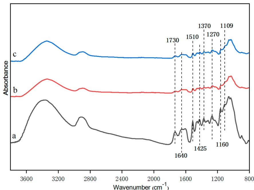
**Figure 1.** Fourier-transform infrared (FTIR) spectra: (a) untreated radiata pine (RP), (b) sodium bicarbonate-treated RP, (c) ozone-treated RP.
