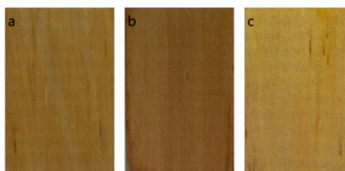
**Figure 4.** Images of surfaces of RP. (a) untreated sample, (b) sodium bicarbonate-treated sample, (c) ozone-treated sample.
