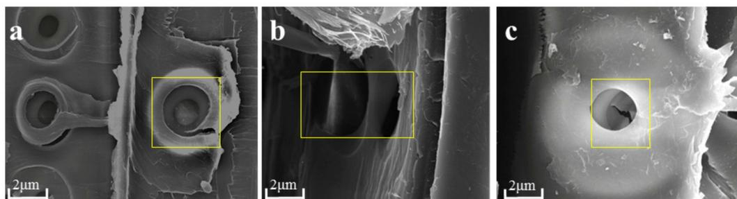
**Figure 5.** SEM images of RP: (a) untreated sample, (b) sodium bicarbonate-treated sample, (c) ozone-treated sample.
