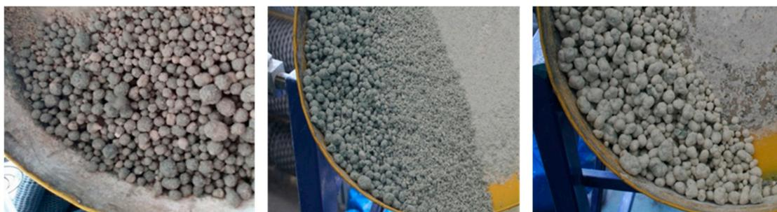
**Figure 2.** The process of granulation of tanning shavings in pulp according to methods 2, 4, and 7.
