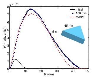
**Figure 5.** The p(r) functions for the initial (solid line) and 150 min solutions (blue triangles) calculated using the Fourier transform method. The p(r) function calculated for a triangular model prism (red dashed line) is shown for comparison. The model is shown in the inset.
