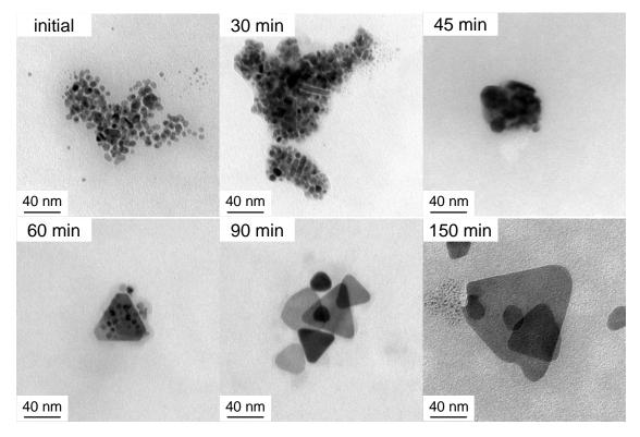
**Figure 1.** Examples of cryo-TEM images as a function of irradiation time. From left to right: Initial 0 min, 30 min, and 45 min (upper row) and 60 min, 90 min and 150 min irradiated solutions (lower row).
