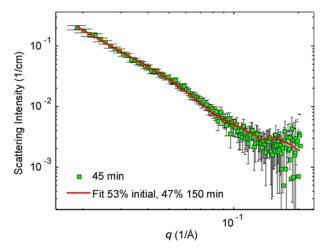
**Figure 7.** The scattering pattern of the 45 min sample (green squares). The solid red line is the corresponding "bimodal" model fit with the contribution of 53% of initial and 47% initial sample. See text for details.
