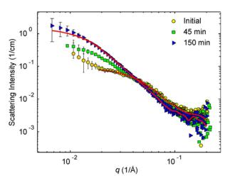
**Figure 3.** SAXS patterns from initial (yellow circles), 45 min (green squares) and 150 min solutions (blue triangles). Solid lines are the corresponding GNOM fits (see Section 3 for details).
