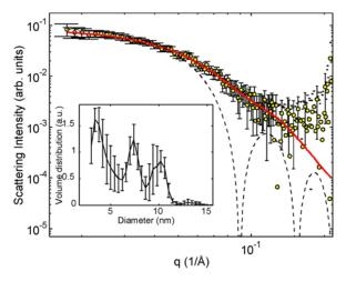
**Figure 6.** The scattering pattern of initial sample (yellow symbols) and theoretical scattering from a sphere with a diameter of 10 nm (dashed line). The inset shows the Monte Carlo (MC) simulated volume distribution of spheres in arbitrary units. It corresponds to the fit (full red line). See text for details.
