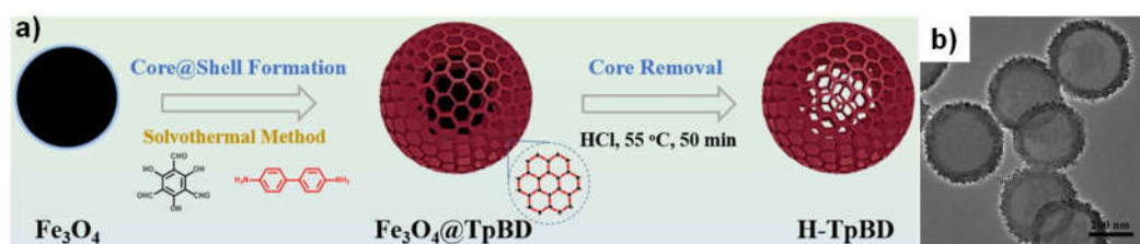
Figure 15. (a) Schematic illustration of the synthesis protocols and chemical structures of the H-TpBD. (b) TEM image of the synthesized H-TpBD. Reprinted with permission from [77]. Copyright (2018) Elsevier B.V.
