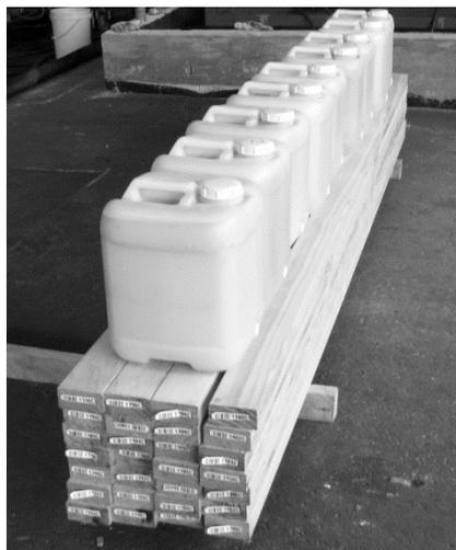
**Figure 2.** Result of a dewatering experiment using 0.105 m<sup>3</sup> of green radiata pine timber. The nine 20-litre containers atop the wood stack store the volume of sap recovered from seven carbon dioxide supercritical fluid to gas phase-change cycles. The wood stack was allowed to passively dry over 2 days from 40% moisture content to ambient equilibrium moisture content, <ca. 20%. Photo: R. Franich (13 August 2008).
