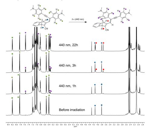
**Figure 5.**  $^{1}$ H-NMR Spectra (toluene- $d_{8}$ , 500 MHz) of **9** recorded after various times of irradiation (440 nm).
