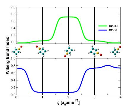
**Figure 4.** Evolution of the C2-C3 and C2-S9 bonds along an entire cycle of Dewar rearrangements, as depicted in Scheme 3 for S-oxide perfluorotetramethylthiophene.
