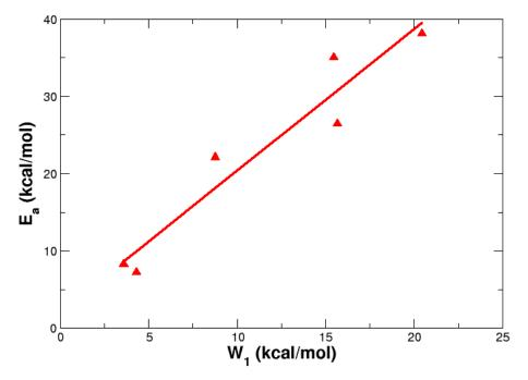
**Figure 2.** Correlation between activation energies and  $W_1$ , the work needed to take the reacting system to the coordinate of the activated reactants:  $W_1(\xi_R \to \xi_{R*}) = -\int_{\xi_{R*}}^{\xi_R} F(\xi) d\xi$ . Linear regression equation:  $E_a = 2.0637 + 1.8327 W_1$ ,  $R^2 = 0.923$ .
