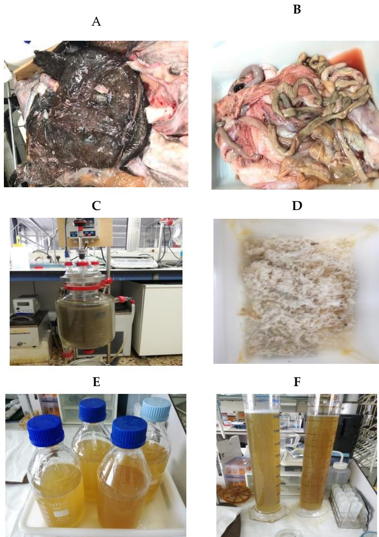
**Figure 1.** Pictures of monkfish substrates and hydrolysates: A) heads, B) viscera, C) Alcalase hydrolysis of monkfish wastes in a 5L-pH-stat reactor, D) clean bones recovered, E) head liquid FPH, and F) viscera liquid FPH.
