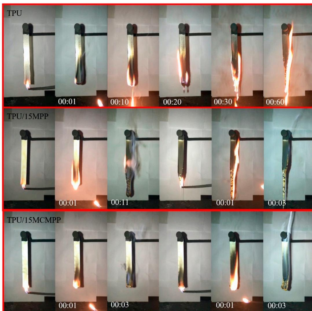
**Figure 4.** Video screenshots of TPU (thermoplastic polyurethane), TPU/MPP (thermoplastic polyurethane containing 15 wt. % of melamine polyphosphate) and TPU/MCMPP (thermoplastic polyurethane containing 15 wt. % of melamine polyphosphate microencapsulated by toluene diisocyanate crosslinked carboxymethyl chitosan) composites during UL-94 testing. Reprinted with permission from [32]. Copyright 2019, Elsevier.
