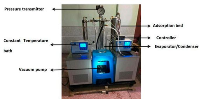
Figure 16. Adsorption refrigeration system performance test device.
