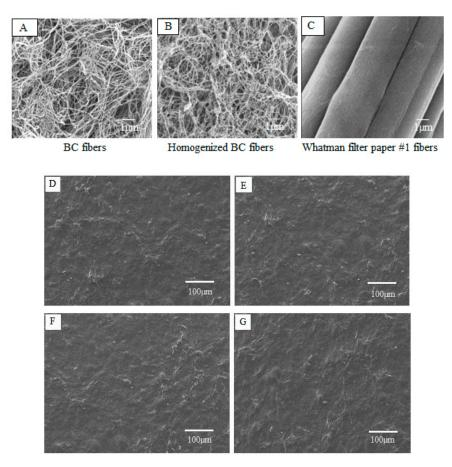
**Figure 1.** SEM images of: (**A**) BC fibers; (**B**) mechanically-disintegrated BC fibers; and (**C**) Whatman filter paper No. 1 fibers at 10,000× magnification. Surface morphology of: (**D**) BCAGG-C1; (**E**) BCAGG-C2; (**F**) BCAGG-C3; and (**G**) BCAGG-C4.
