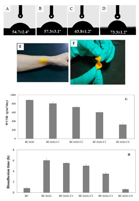
**Figure 4.** Water contact angles of: (**A**) BCAGG-C1; (**B**) BCAGG-C2; (**C**) BCAGG-C3; and (**D**) BCAGG-C4; (**E**) film attachment to skin; (**F**) film flexibility; (**G**) WVTR; and (**H**) bioadhesion time.
