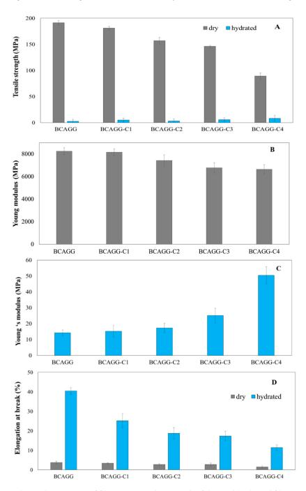
**Figure 5.** Mechanical properties of films: (**A**) tensile strength of dry and hydrated films; (**B**) Young's modulus of dry films; (**C**) Young's modulus of hydrated films; and (**D**) elongation at break (%) of dry and hydrated films.
