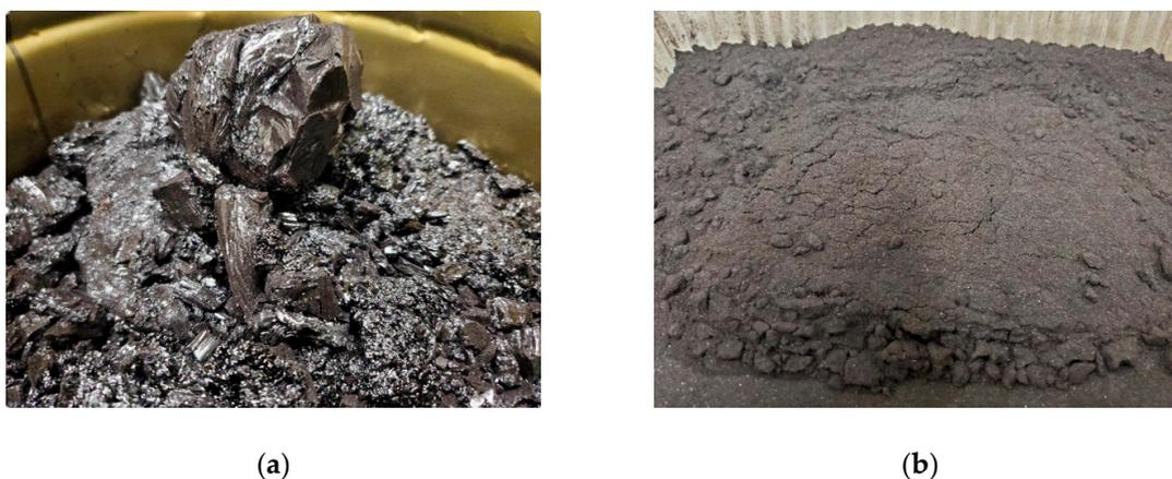
**Figure 1.** Asphaltenes: (a) solid form; (b) powder form after passing through a #100 sieve.
