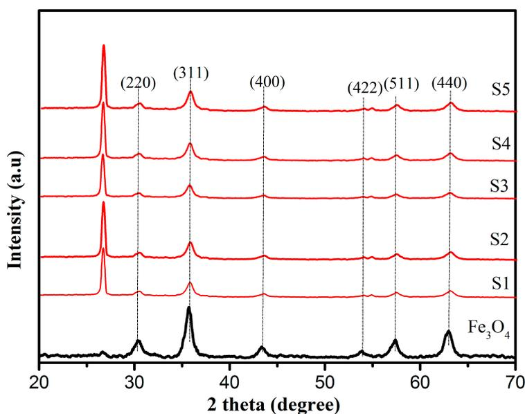
Figure 1. X-ray diffraction (XRD) patterns of Fe $_3$ O $_4$ , S1, S2, S3, S4, and S5.
