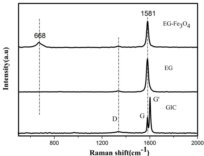
**Figure 5.** Raman spectra of graphite, graphene intercalation compounds (GIC), EG and EG/ $\text{Fe}_3\text{O}_4$  composite.
