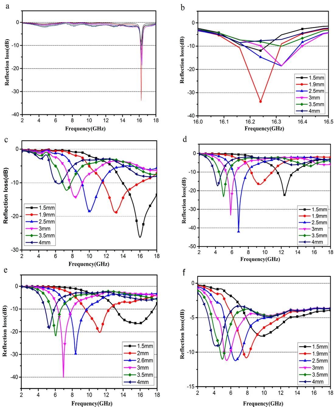
**Figure 10.** The calculated  $R_L$  for S1 (a,b), S2 (c), S3 (d), S4 (e) and S5 (f) with different thicknesses in the frequency range of 2–18 GHz.
