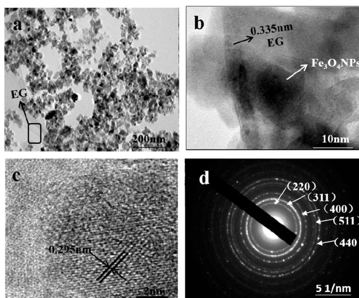
**Figure 3.** Transmission electron microscopy (TEM) images of EG/Fe<sub>3</sub>O<sub>4</sub> (S1) composite (a); High Resolution Transmission Electron Microscope (HRTEM) image (b,c) and Selected Area Electron Diffraction (SAED) pattern (d) of EG/ Fe<sub>3</sub>O<sub>4</sub> (S1) composite.
