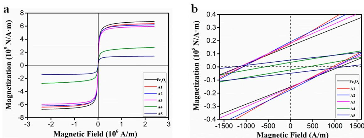
**Figure 7.** The magnetization curves of Fe<sub>3</sub>O<sub>4</sub> and EG/ Fe<sub>3</sub>O<sub>4</sub> (a) and an expanded view of the low-field magnetization curves (b).
