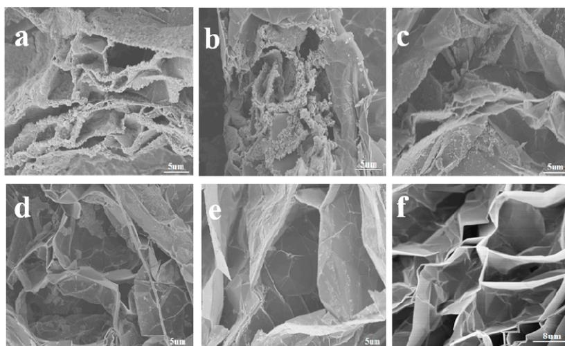
**Figure 2.** Scanning electron microscopy (SEM) images of expanded graphite (EG)/Fe<sub>3</sub>O<sub>4</sub> prepared from different concentrations of Fe<sub>3</sub>O<sub>4</sub> (gradually decreased from (a–e) in the figure) and EG (f), respectively.
