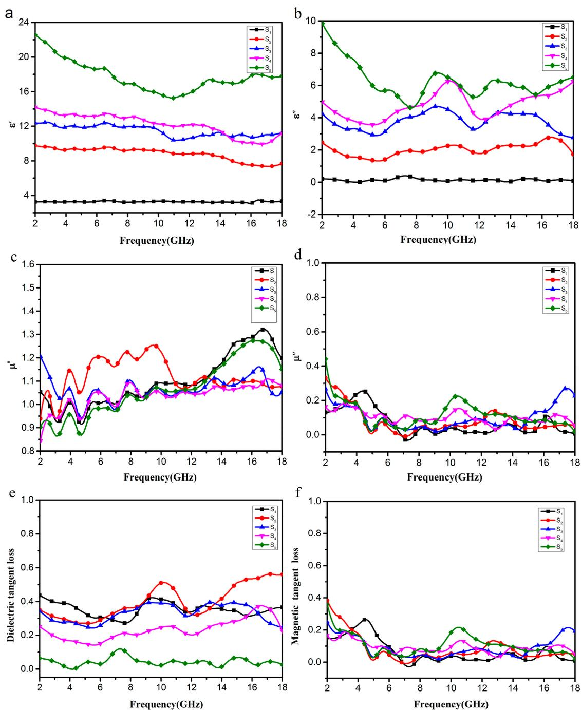
**Figure 9.** Frequency dependence on real parts (a) and imaginary parts (b) of the complex permittivity, real parts (c) and imaginary parts (d) of the complex permeability, and the corresponding dielectric loss tangents (e) and magnetic loss tangents (f) of composites S1–S5.
