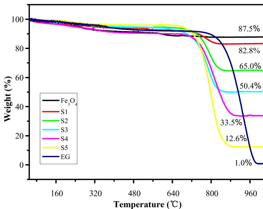
**Figure 8.** Thermogravimetric (TG) curves of Fe<sub>3</sub>O<sub>4</sub> and composites S1–S5 under air atmosphere.
