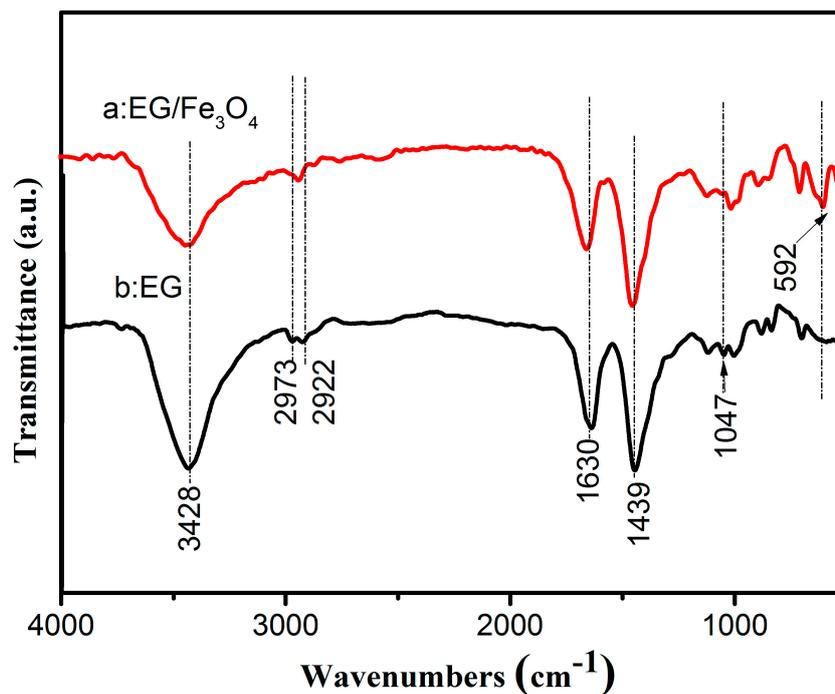
Figure 4. Fourier transform infrared (FT-IR) spectra of EG and EG/Fe<sub>3</sub>O<sub>4</sub> composites.
