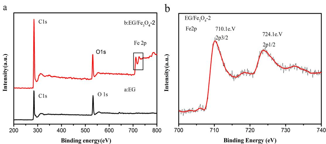
**Figure 6.** X-ray photoelectron spectroscopy (XPS): (a) wide scan, (b) Fe 2p spectrum of the EG/ $\text{Fe}_3\text{O}_4$  composite.
