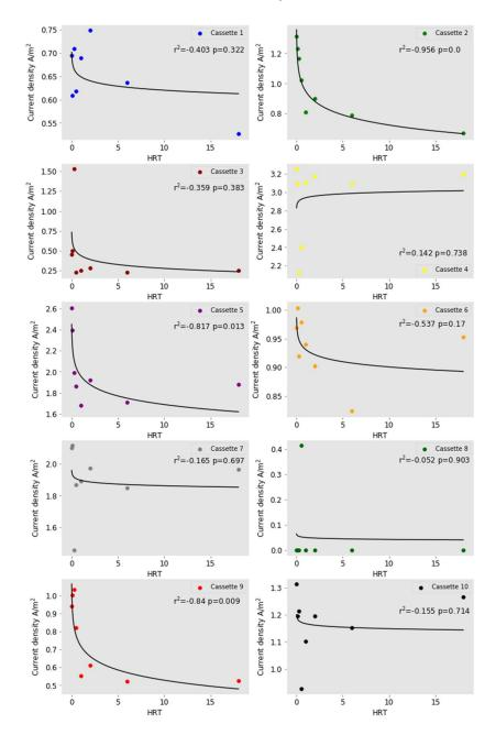
Figure S1. The average current densities compared to HRT for the 10-cassette style electrodes.
