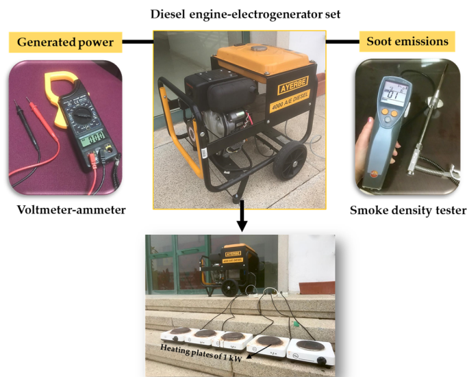
Figure 5. Schematic summary of mechanical and environmental characterization of diesel engine-electrogenerator set.
