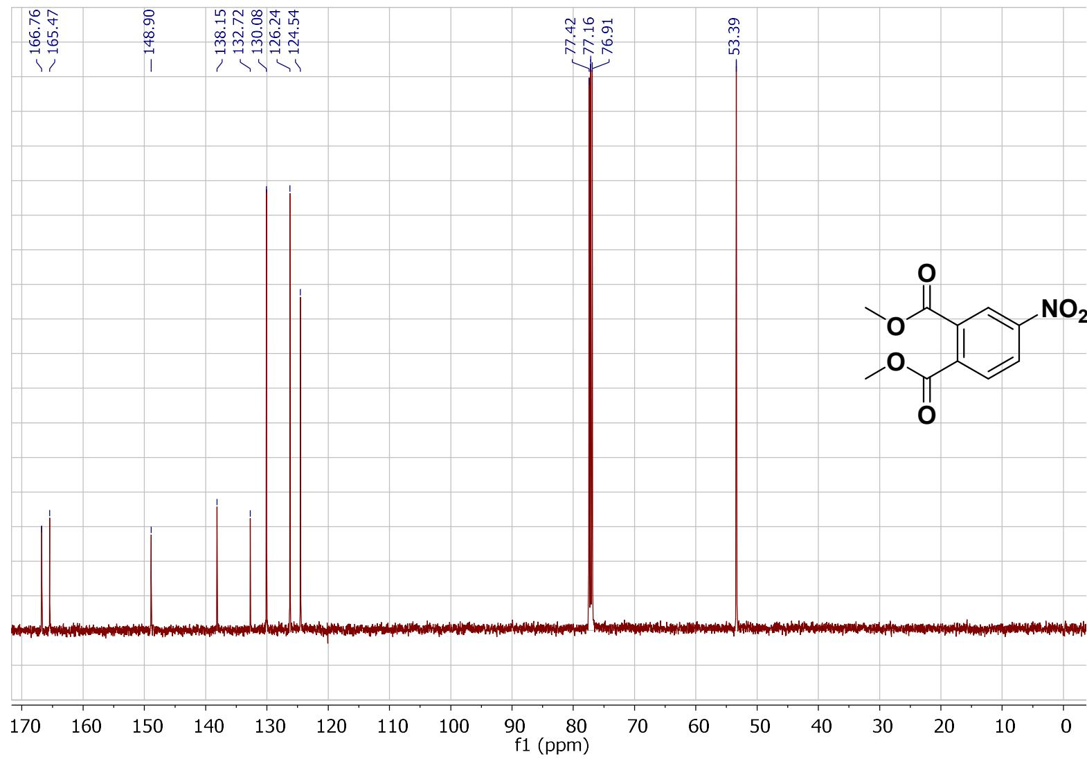
Figure S57. <sup>13</sup>C-NMR spectrum for dimethyl 4-nitrophthalate (**5b**).
