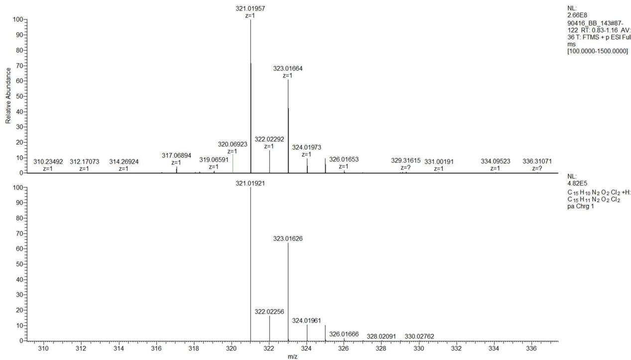
**Figure S95.** HRMS spectrum for 8,9-dichloro-5-methyl-5,12-dihydrodibenzo[b,f][1,4]diazocine-6,11-dione (**3g**).
