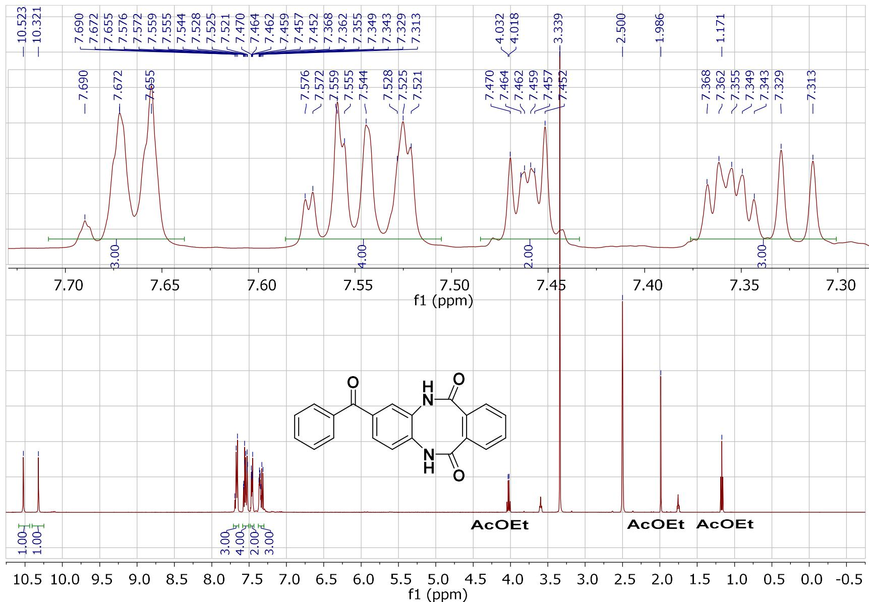
**Figure S10.**  $^1\text{H-NMR}$  spectrum for 2-benzoyl-5,12-dihydrodibenzo[*b,f*][1,4]diazocine-6,11-dione (**3c**).
