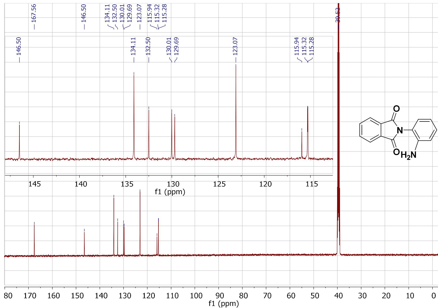
Figure 54. <sup>13</sup>C-NMR spectrum for 2-(2-aminophenyl)isoindoline-1,3-dione (10).
