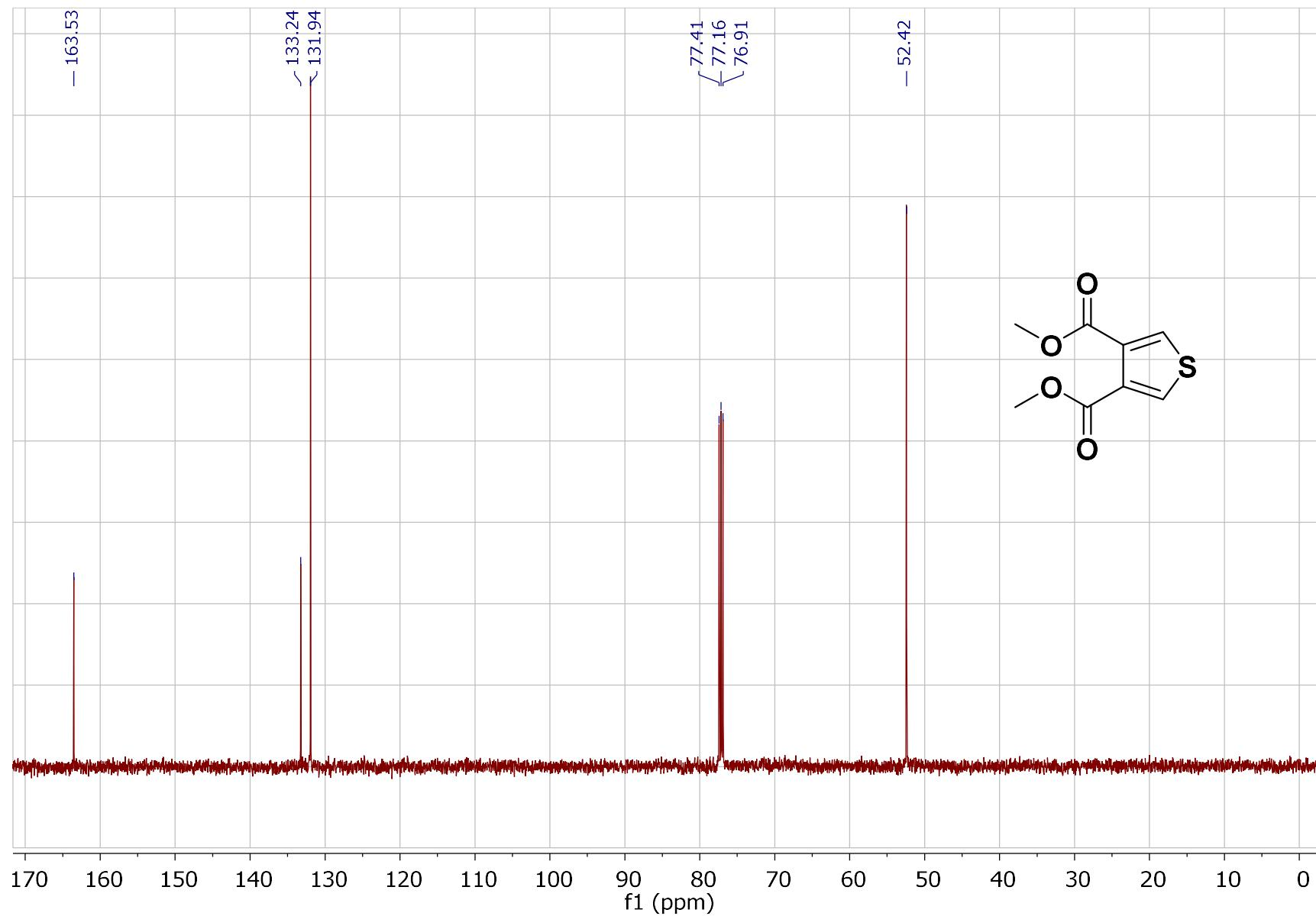
Figure S60. <sup>13</sup>C-NMR spectrum for dimethyl thiophene-3,4-dicarboxylate (5e).
