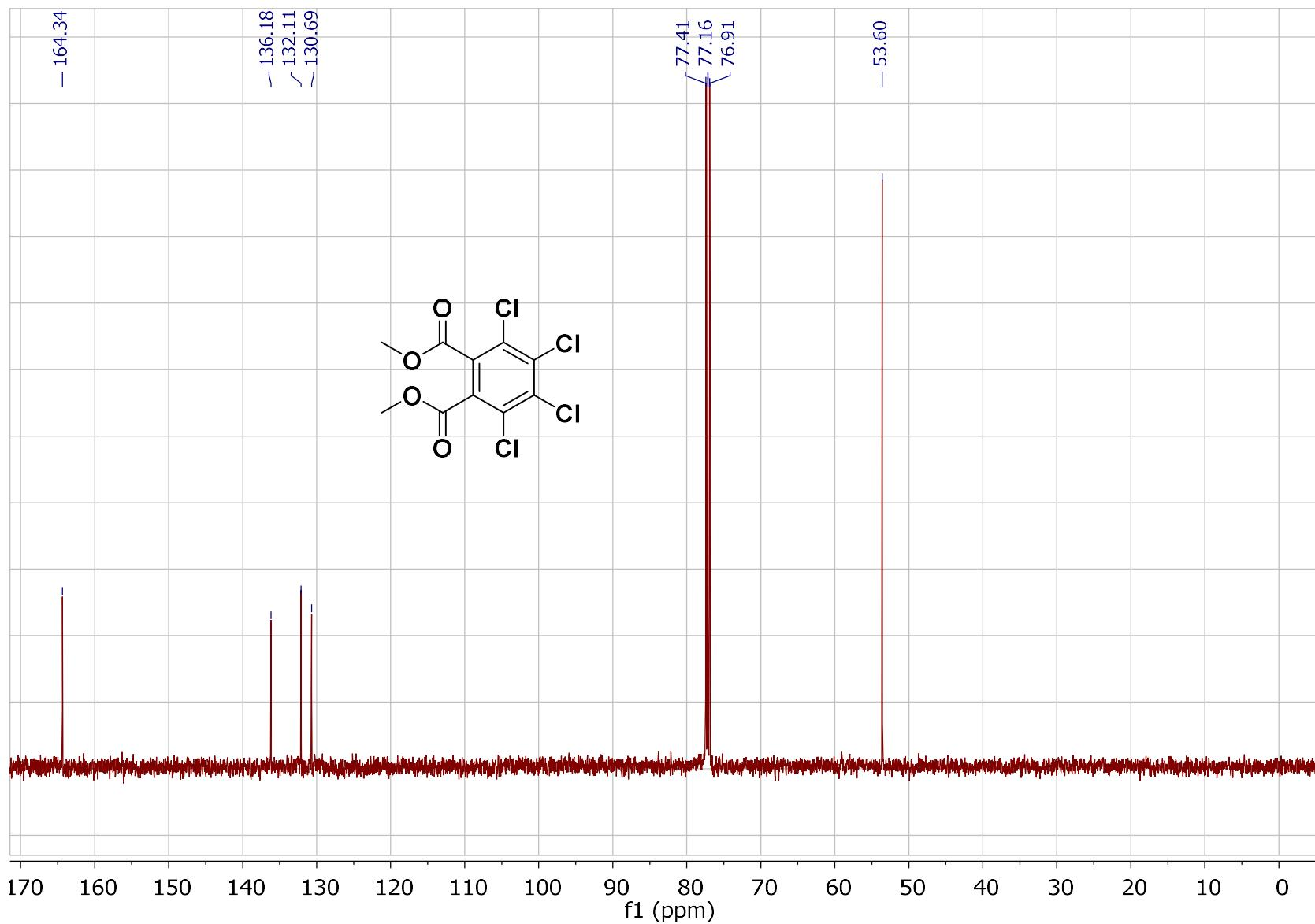
Figure S59.  $^{13}\text{C}$ -NMR spectrum for dimethyl 3,4,5,6-tetrachlorophthalate (**5d**).
