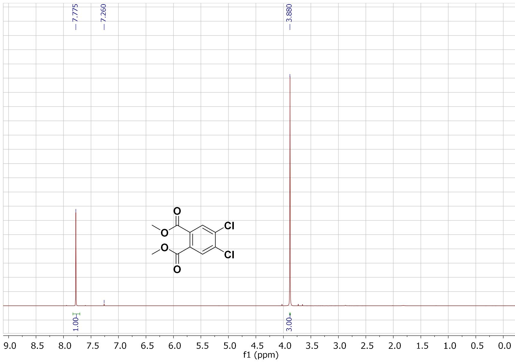
Figure S31. <sup>1</sup>H-NMR spectrum for dimethyl 4,5-dichlorophthalate (**5c**).
