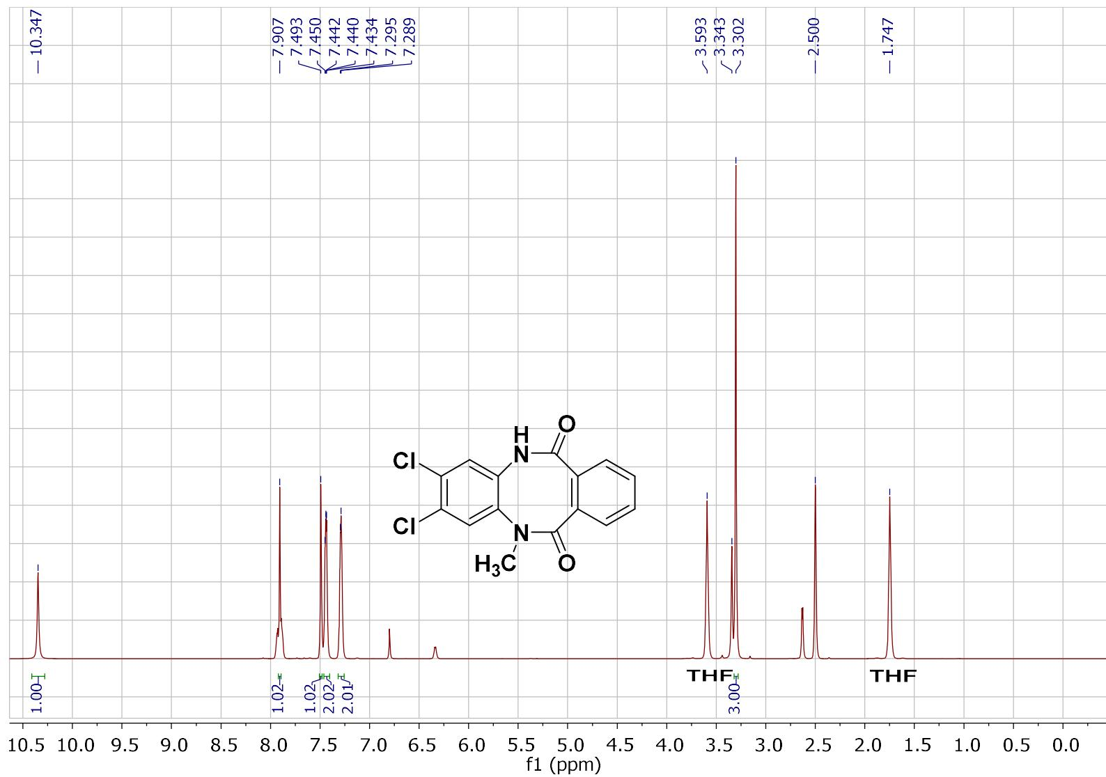
**Figure S13.** <sup>1</sup>H-NMR spectrum for 2,3-dichloro-5-methyl-5,12-dihydrodibenzo[*b,f*][1,4]diazocine-6,11-dione (**3f**).
