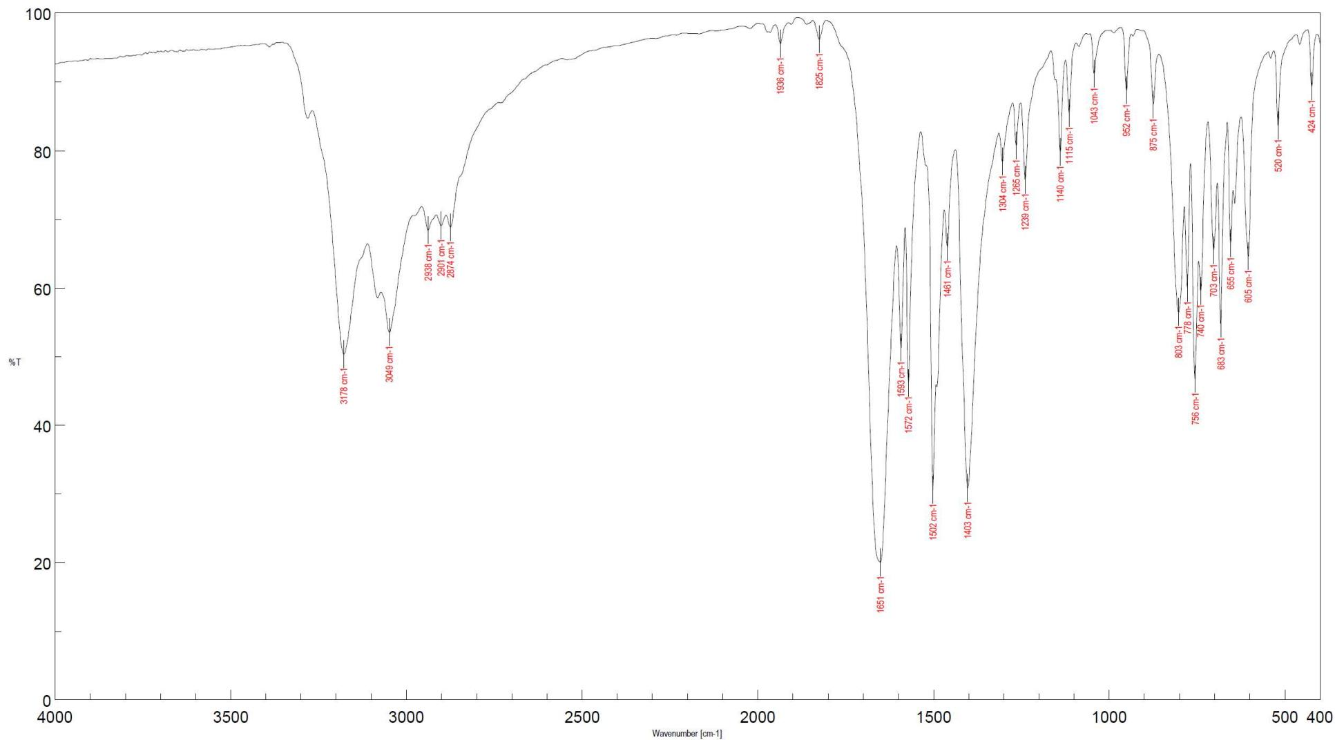
**Figure S116.** IR spectrum for 5,12-dihydronaphthalene[*b,f*][1,4]diazocine–6,11-dione (**3a**).
