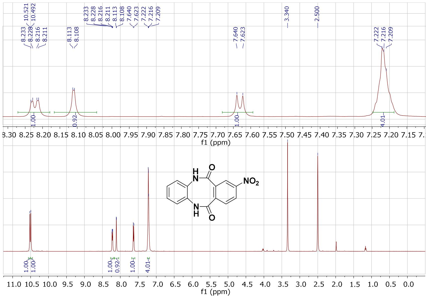
**Figure S11.**  $^1\text{H}$ -NMR spectrum for 8-nitro-5,12-dihydrodibenzo[b,f][1,4]diazocine-6,11-dione (**3d**).
