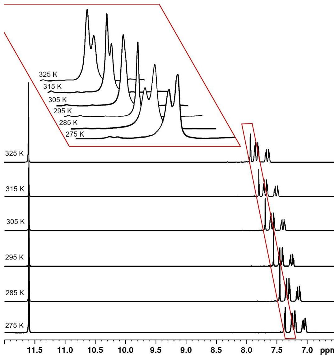
**Figure S25b.** <sup>1</sup>H-NMR spectra for **9b** registered in the temperature range of 275–325 K. The magnified region shows different temperature drift of the two conformers.
