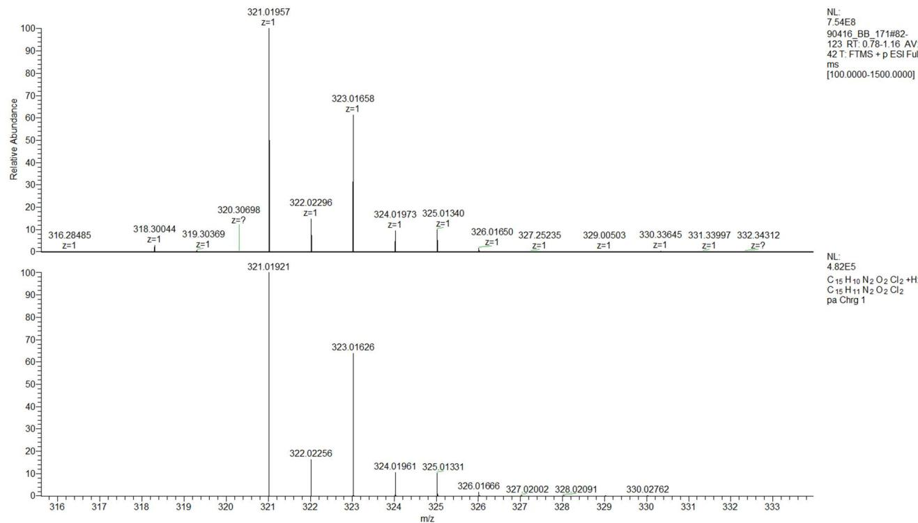
**Figure S94.** HRMS spectrum for 2,3-dichloro-5-methyl-5,12-dihydrodibenzo[b,f][1,4]diazocine-6,11-dione (**3f**).
