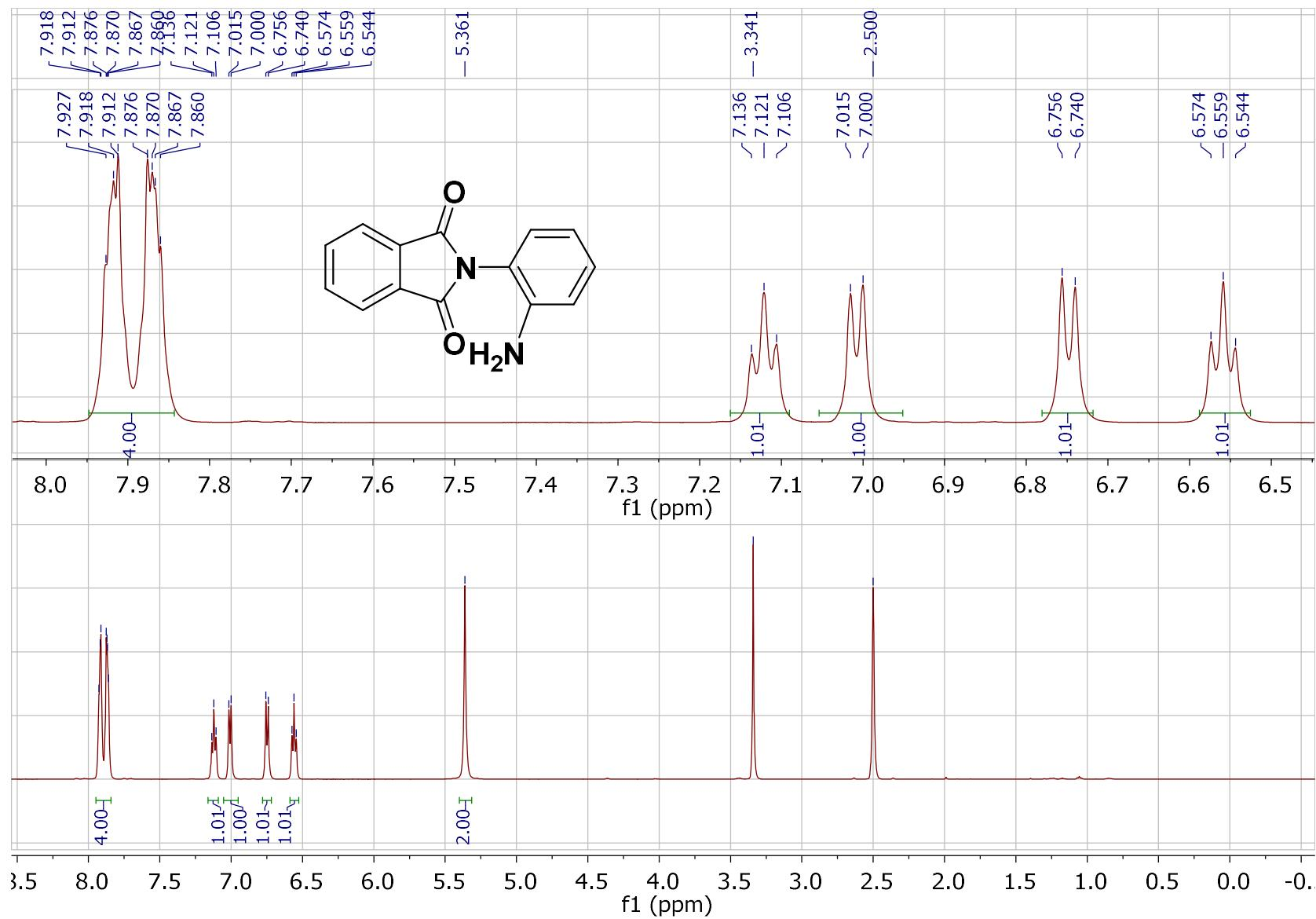
**Figure S27.**  $^1\text{H}$ -NMR spectrum for 2-(2-aminophenyl)isoindoline-1,3-dione (**10**).
