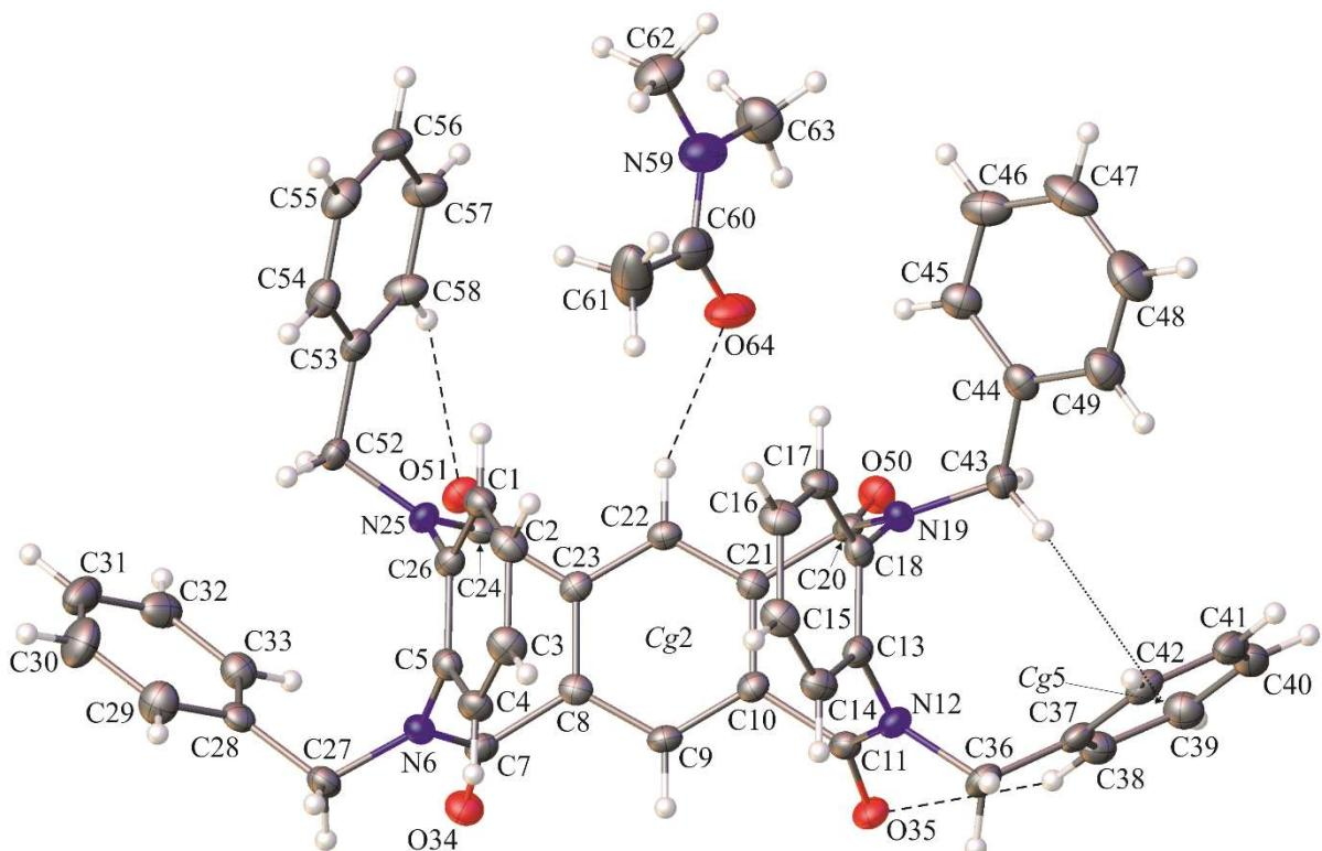
**Figure S4.** Asymmetric unit of the crystal lattice of **9c** with crystallographic atom numbering. Displacement ellipsoids are drawn at the 50% probability level. The H-atoms are shown as small
