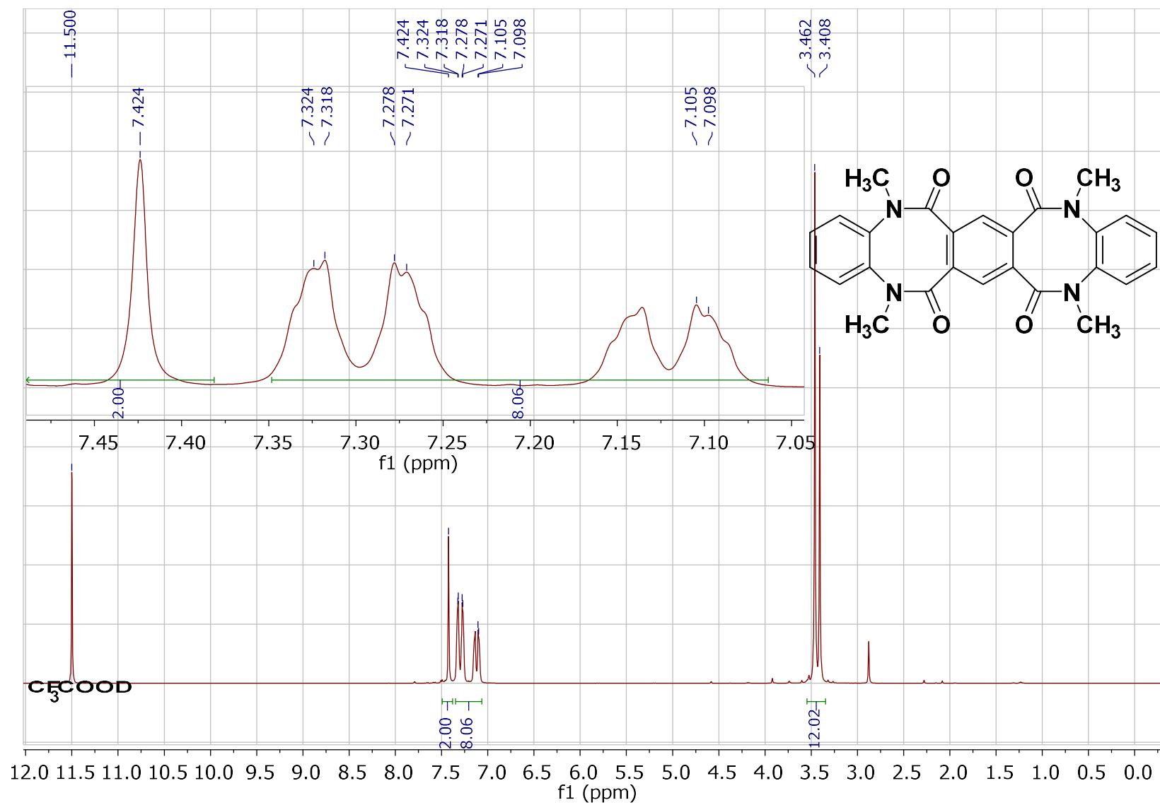
Figure S25a. <sup>1</sup>H-NMR spectrum for **9b** (registered in 295 K).
