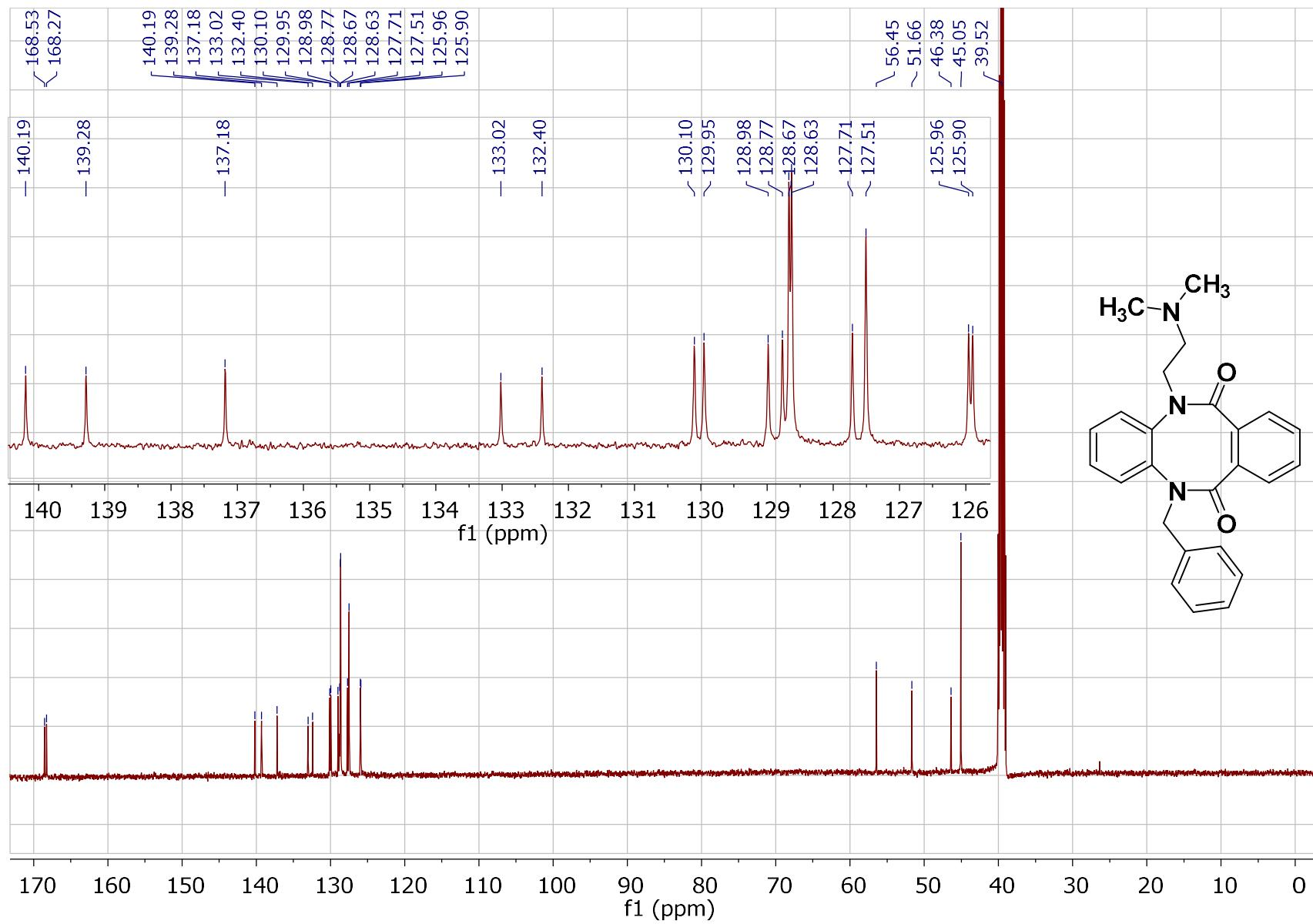
**Figure S47.**  $^{13}\text{C}$ -NMR spectrum for 5-benzyl-12-(2-(dimethylamino)ethyl)-5,12-dihydrodibenz[b,f][1,4]diazocine-6,11-dione (**3m**).
