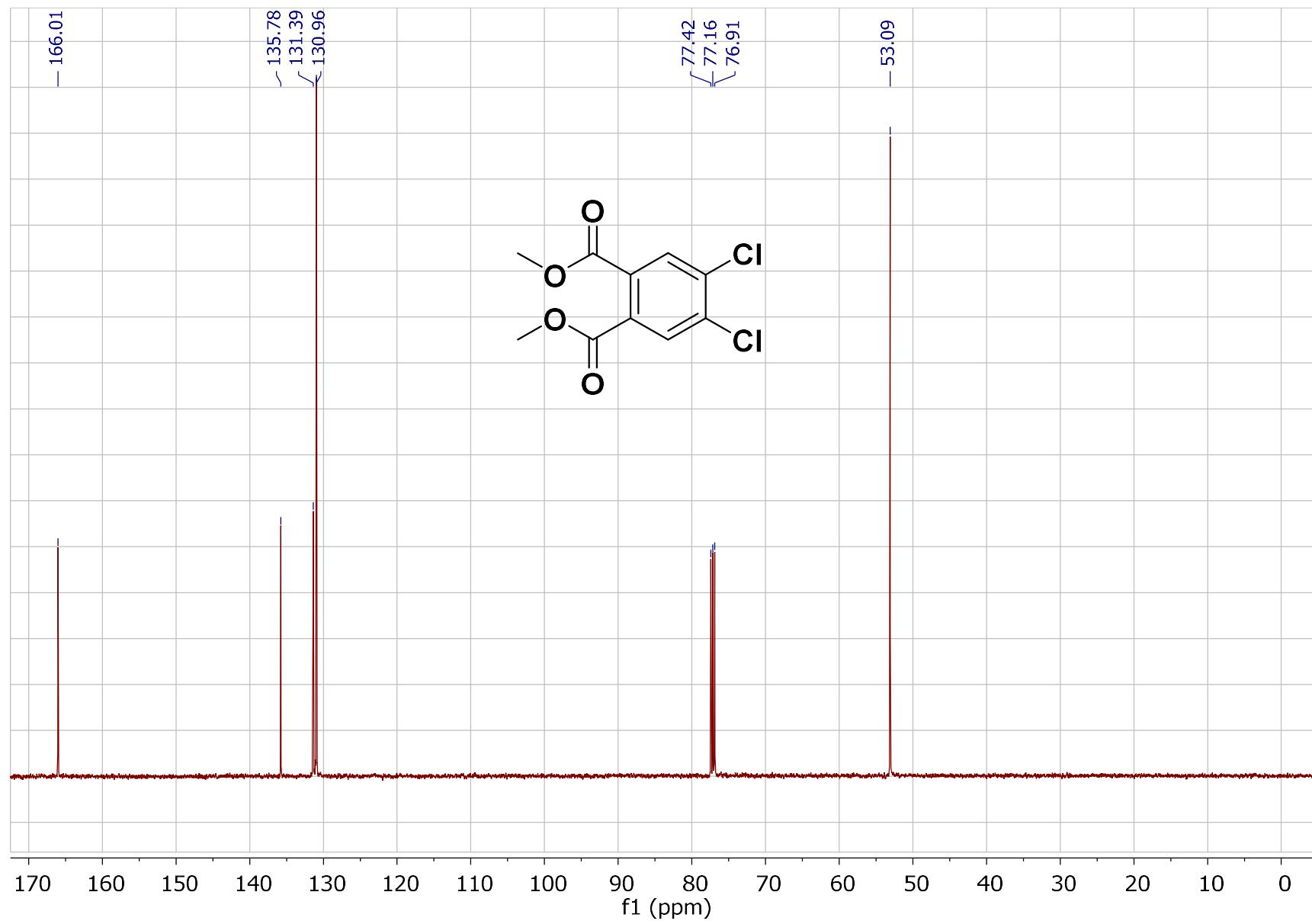
Figure S58. <sup>13</sup>C-NMR spectrum for dimethyl 4,5-dichlorophthalate (**5c**).
