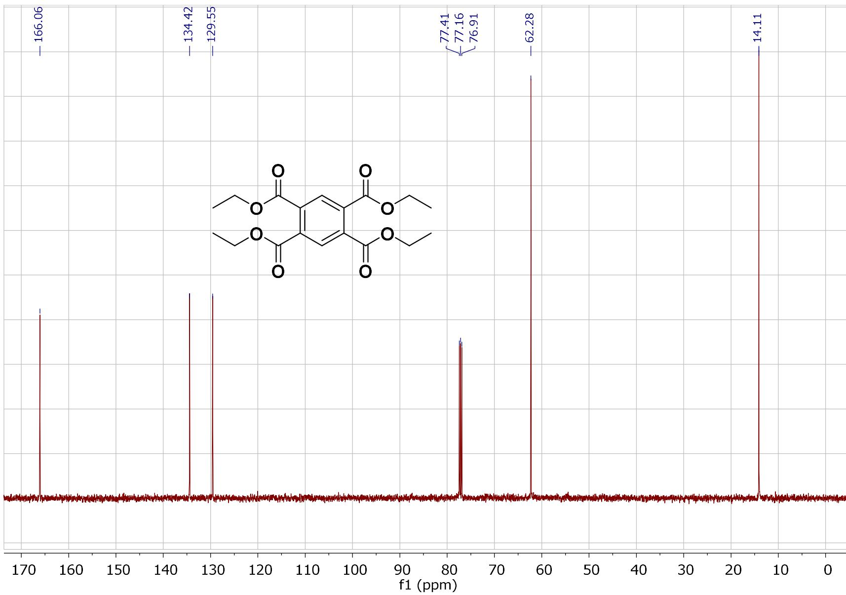
Figure S61.  $^{13}\text{C}$ -NMR spectrum for tetraethyl benzene-1,2,4,5-tetracarboxylate (8).
