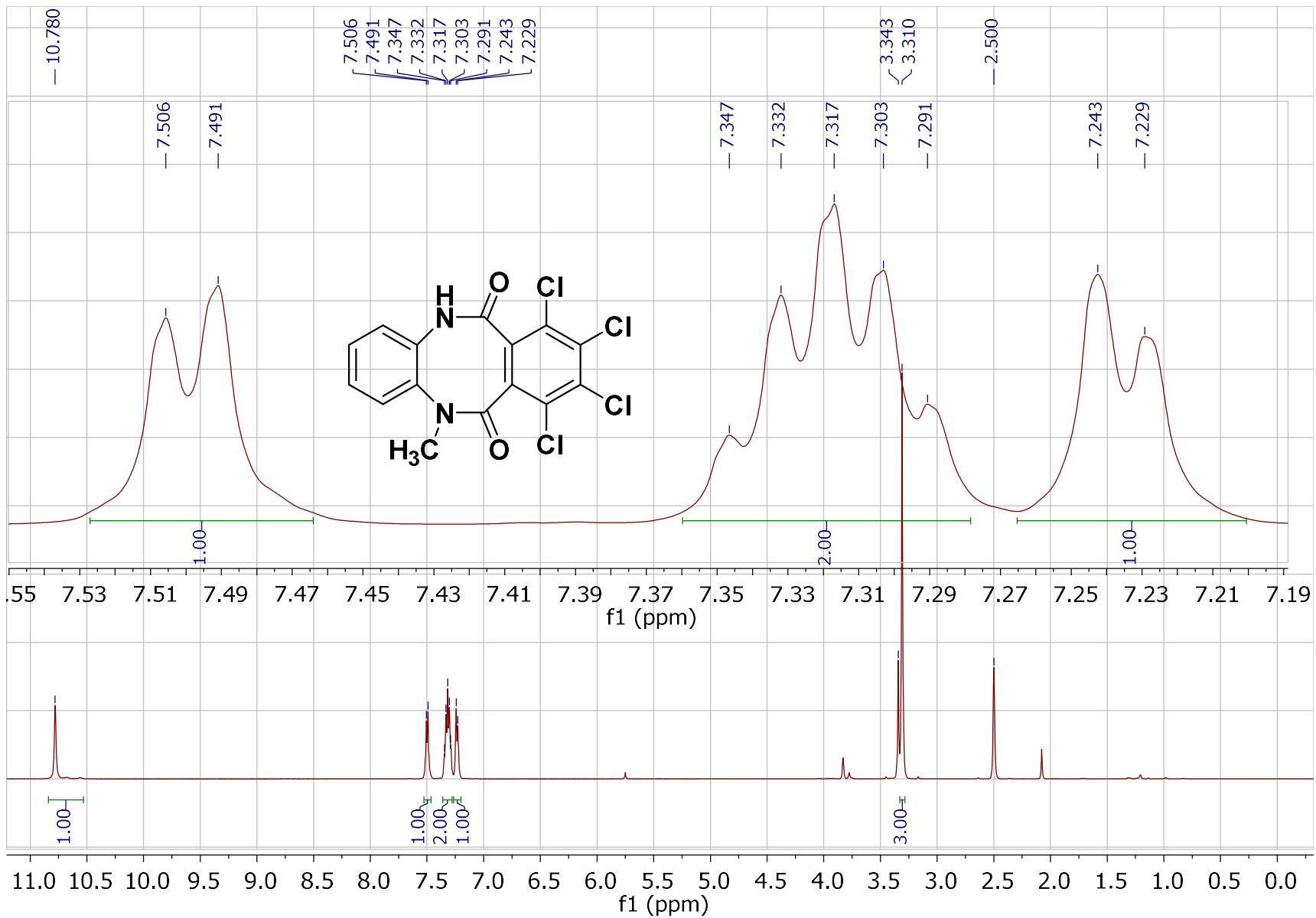
**Figure S15.** <sup>1</sup>H-NMR spectrum for 7,8,9,10-tetrachloro-5-methyl-5,12-dihydrobenzo[*b,f*][1,4]diazocine-6,11-dione (**3h**).
