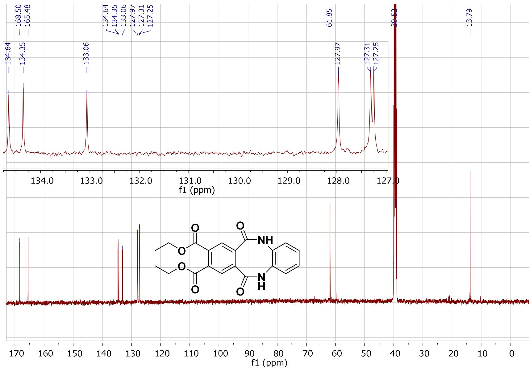
**Figure S45.** <sup>13</sup>C-NMR spectrum for diethyl 6,11-dioxo-5,6,11,12-tetrahydrodibenzo[*b,f*][1,4]diazocine-8,9-dicarboxylate (**3k**).
