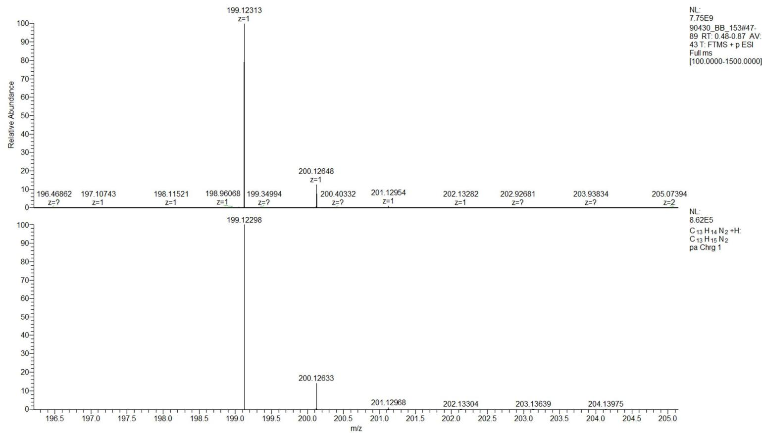
**Figure S110.** HRMS spectrum for  $N^1$ -benzylbenzene-1,2-diamine (**4f**).
