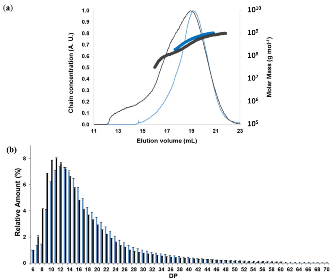
**Figure 2.** Macromolecular structure of native and acetylated waxy maize starch. (a) Elugrams (thin lines) and molar mass distributions (thick lines) of native WMS (blue) and acetylated WMS (AWMS) after deacetylation (black) obtained by AF4-MALLS; (b) Chain length distributions of WMS (Blue) and AWMS after deacetylation (Black). DS before deacetylation: 2.6.
