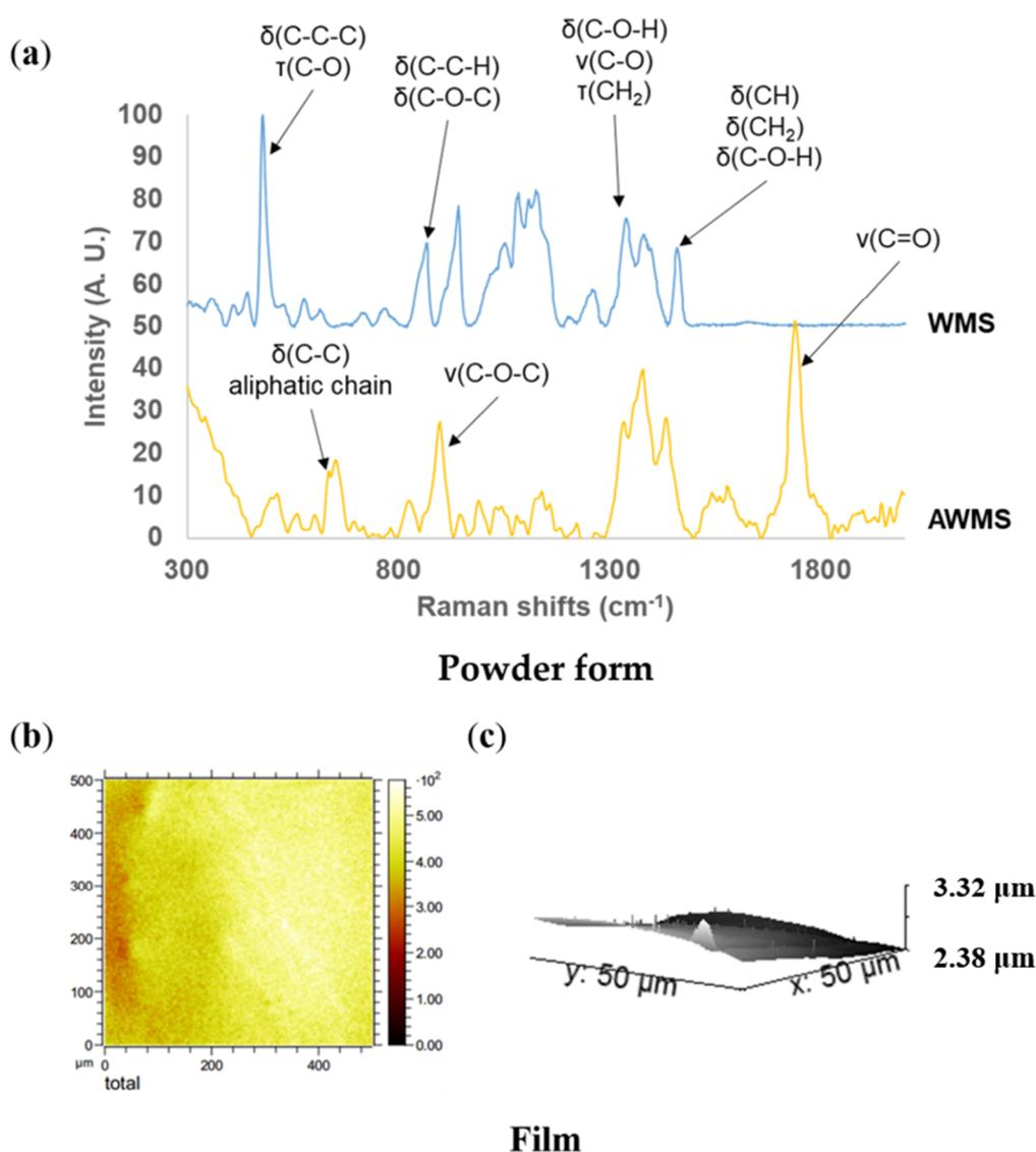
**Figure 4.** Surface characterization of acetylated waxy maize starch (DS 2.6). (a) Raman spectra of WMS and AWMS, (b) TOF-SIMS 2D mapping of the acetate fragment in AWMS, (c) AFM topography image of AWMS.
