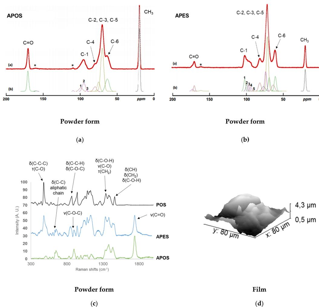
**Figure 7.** Bulk and surface characterization of APES and APOS Solid-state  $^{13}\text{C}$ -NMR spectra obtained for APOS (a) and APES (b) and their spectral decomposition, Raman spectra of POS, APOS and APES (c), AFM topography image of APES (d). The DS of APOS and APES before deacetylation were 2.4 and 0.7, respectively. \*Spinning side band.
