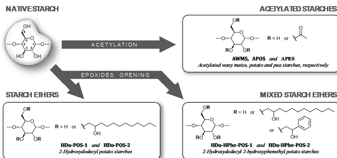
Figure 1. Synthesis, representation and codification of modified starches.
