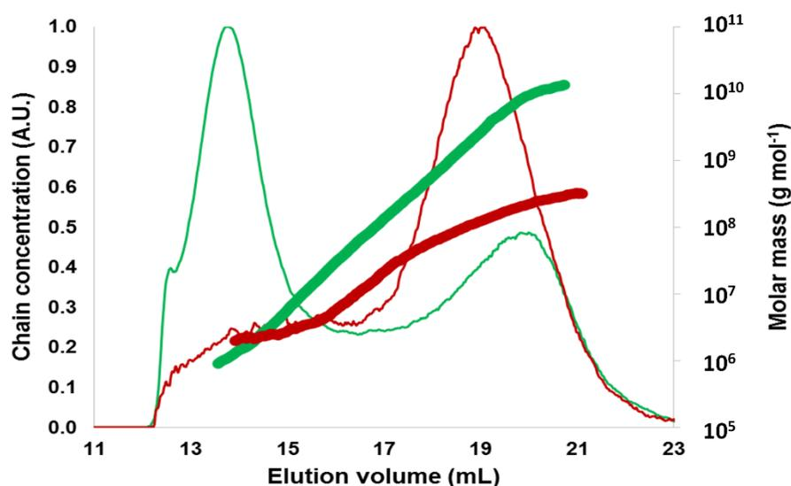
**Figure 8.** Macromolecular characteristics of native and etherified potato starches obtained by AF4-MALLS. Elugrams, i.e., chain concentration versus elution volume (thin lines), and molar mass distributions (thick lines) for POS (dark red), and HDo-POS-1 (green). Native potato (POS) starch and corresponding etherified starch with DS 0.40: HDo-POS-1.
