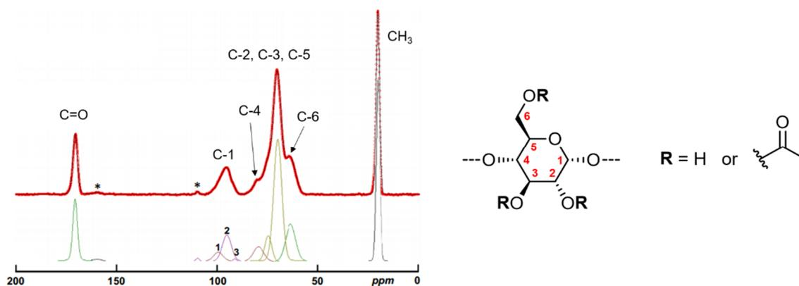
**Figure 3.** Solid-state  $^{13}\text{C}$ -NMR spectrum obtained for acetylated waxy maize starch (DS 2.6) and its spectral decomposition. \* Spinning side band.
