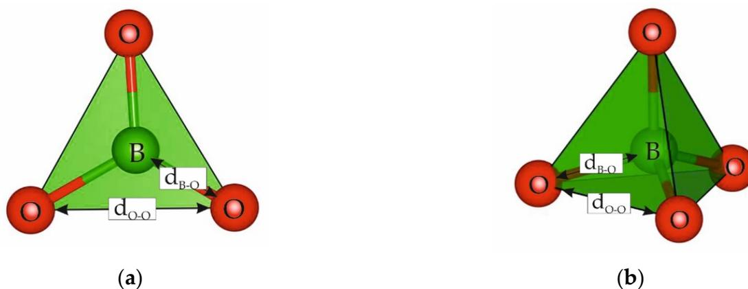
**Figure 2.** FSU in orthoborate structures: (a) isolated  $\text{BO}_3$ -triangles and (b)  $\text{BO}_4$ -tetrahedra.
