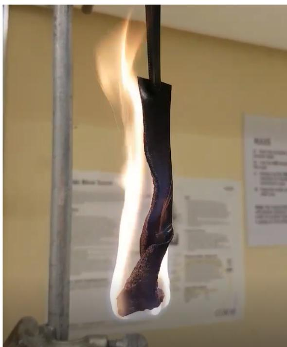
**Figure 4.** The burning behavior of a typical 2CB material sample.
