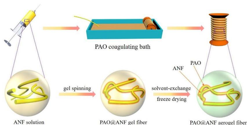
**Scheme 1.** Schematic diagram for the wet spinning of the polyamidoxime aramid nanofiber (PAO@ANF) aerogel fibers.
