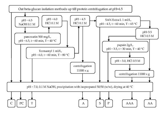
**Figure 1.** β-Glucan purification block-flow diagram. C—control sample, PC—sample after pancreatin digestion, T—sample after treatment with Termamyl SCDS, A—sample acidified to pH 4.5, S—sample treated with SAN Extra L, AA—sample acidified to pH 3.5, P—sample digested with papain, AAA - sample acidified to pH 3.0.
