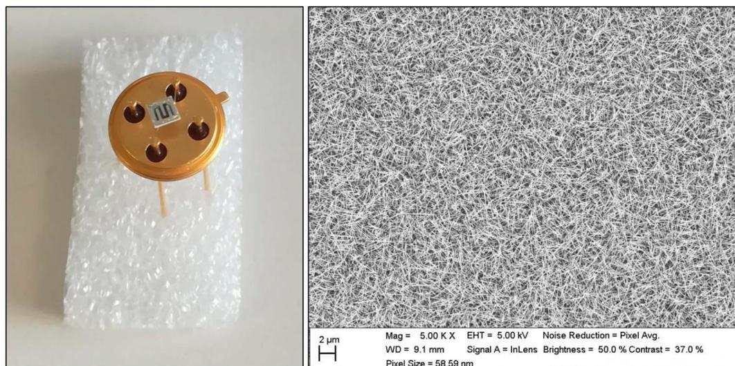
**Figure 5.** On the left, an image of a SnO<sub>2</sub>Au nanowire sensor with its support. On the right, a SEM image of the same sensor where the nanowires are visible.
