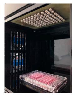
**Figure 5.** Photograph of the illumination device (left) and the  $10 \times 8$  blue LED array (right).
