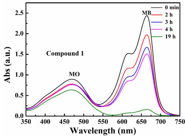
**Fig. S31.** The selective adsorption capability of compound 1 toward the mixed dyes: MO and MB.
