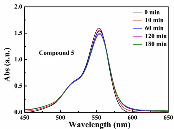
**Fig. S40.**Compound 5 was used to adsorb RhB aqueous solution
