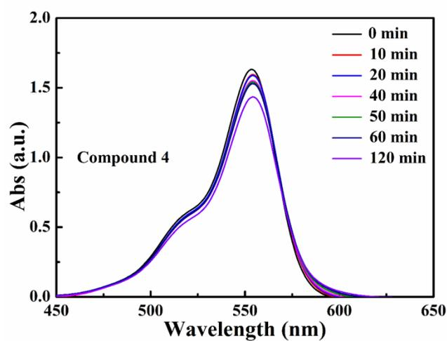
**Fig. S39.**Compound 4 was used to adsorb RhB aqueous solution
