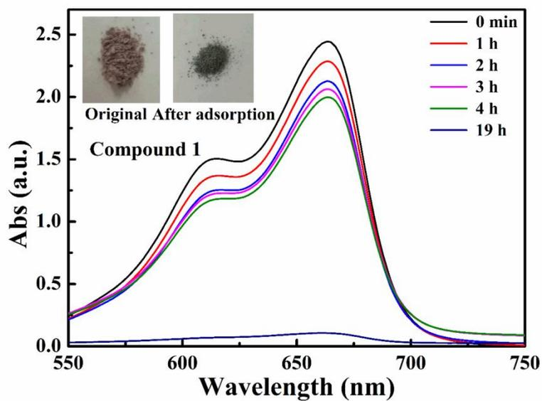
**Fig. S15.** Compound 1 was used to adsorb MB (10 mg/L, 100 mL) aqueous solution
