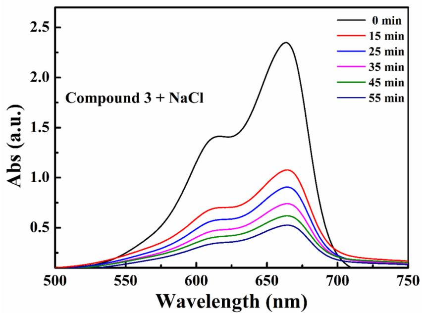
**Fig. S52.**Compound 3 was used to adsorb MB+NaCl aqueous solution
