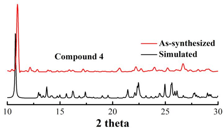
**Fig. S6.** Simulated and experimental XRD spectra of compound 4. Due to the moisture absorption of DMF, partial crystal structures decomposed.
