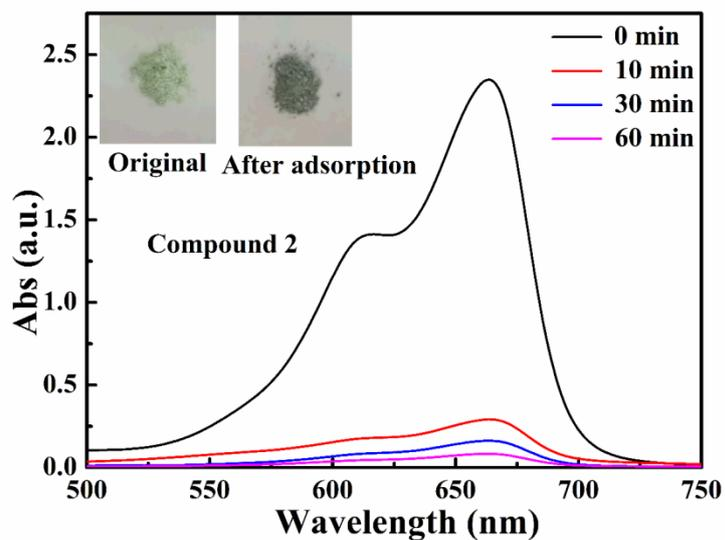
**Fig. S16.**Compound 2 was used to adsorb MB (10 mg/L, 100 mL) aqueous solution
