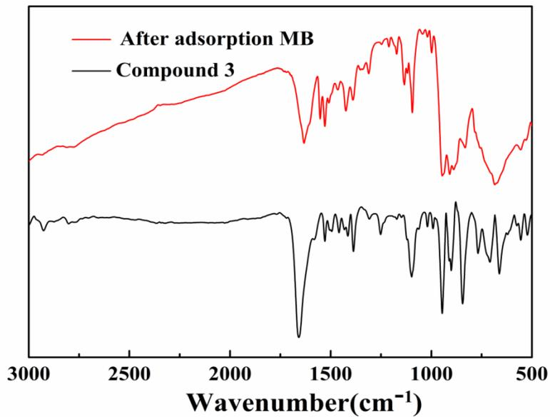
**Fig. S22.** IR spectra of the final recycled powdered solid and compound 3.
