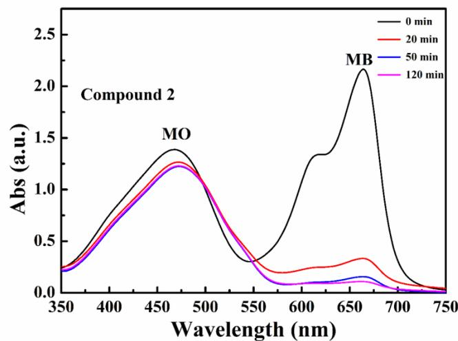
**Fig. S32.** The selective adsorption capability of compound 2 toward the mixed dyes: MO and MB.
