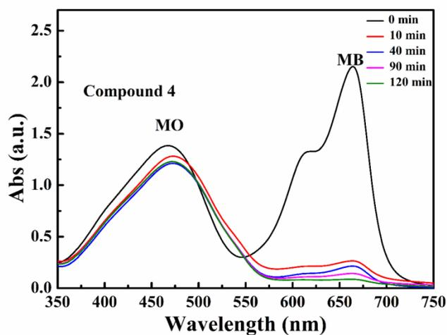
**Fig. S34.** The selective adsorption capability of compound **4** toward the mixed dyes: MO and MB.
