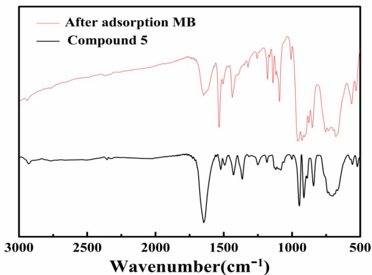
**Fig. S24.** IR spectra of the final recycled powdered solid and compound 5.
