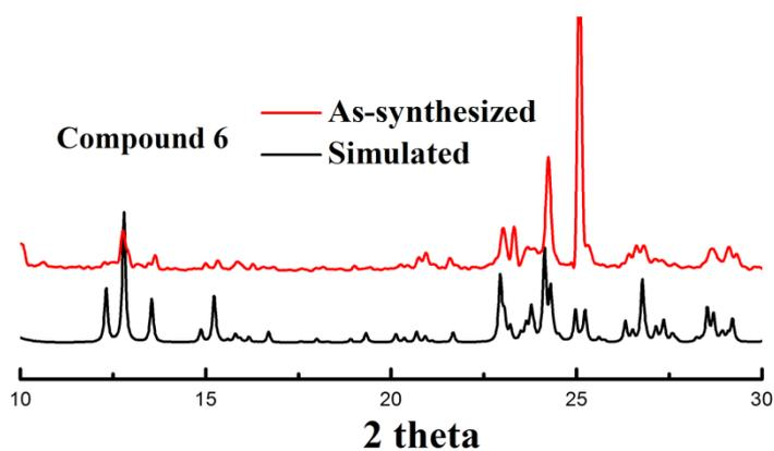
**Fig. S8.** Simulated and experimental XRD spectra of compound 6
