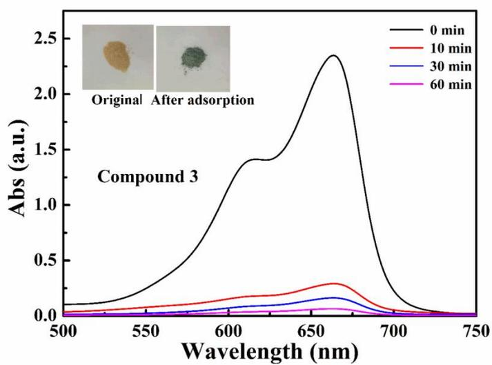
**Fig. S17.**Compound 3 was used to adsorb MB (10 mg/L, 100 mL) aqueous solution
