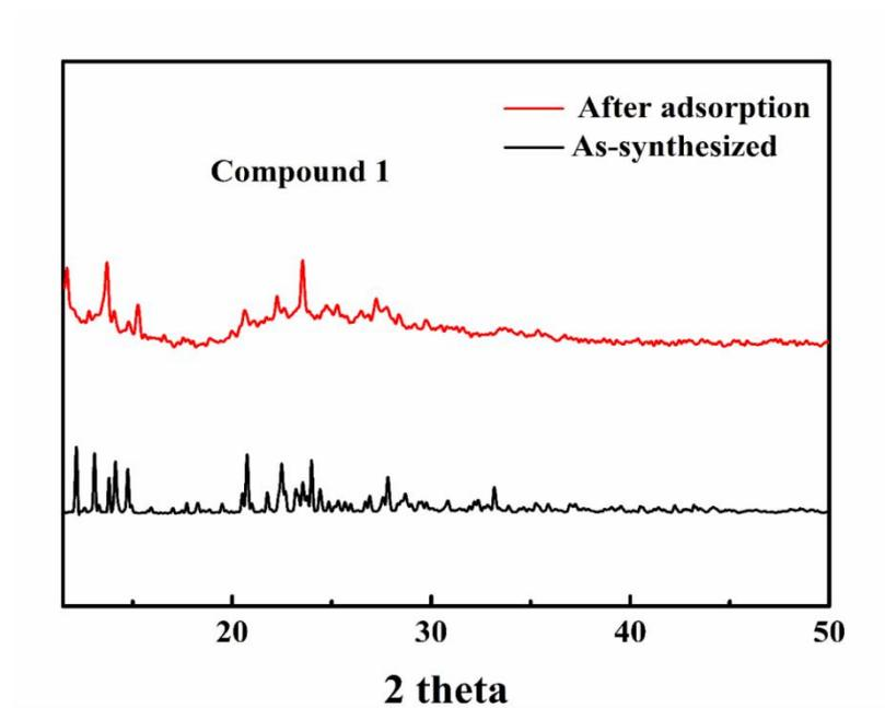
**Fig. S47.** Experimental and after adsorption XRD spectra of compound 1
