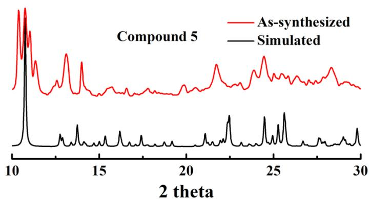
**Fig. S7.** Simulated and experimental XRD spectra of compound 5. Due to the moisture absorption of DMF, partial crystal structures decomposed.
