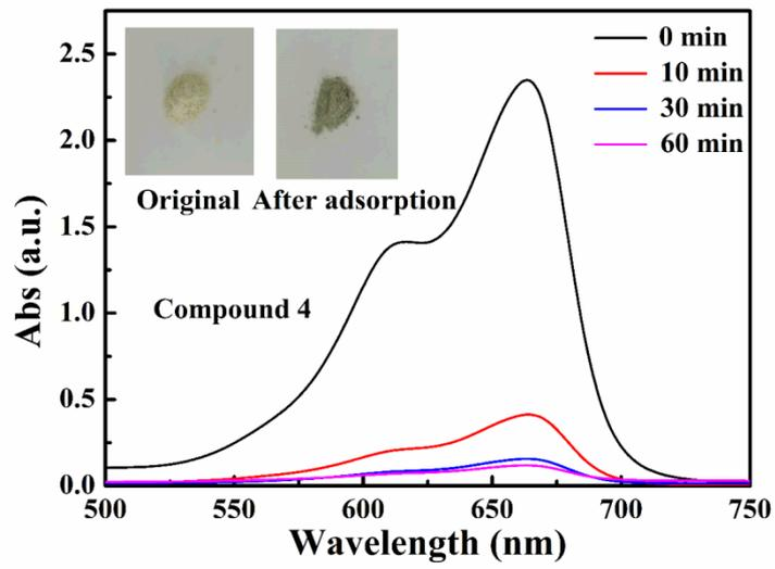
**Fig. S18.**Compound 4 was used to adsorb MB (10 mg/L, 100 mL) aqueous solution
