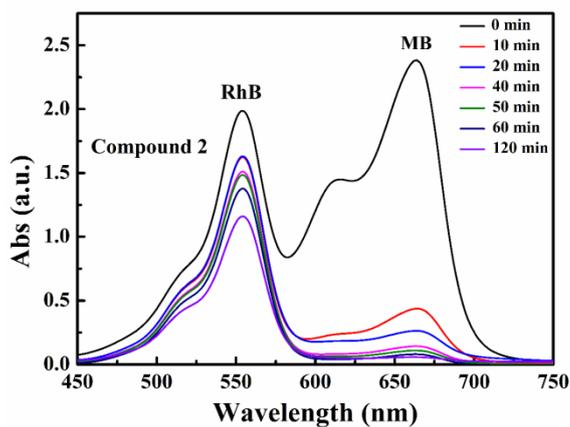
**Fig. S27.** The selective adsorption capability of compound **2** toward the mixed dyes: RhB and MB.
