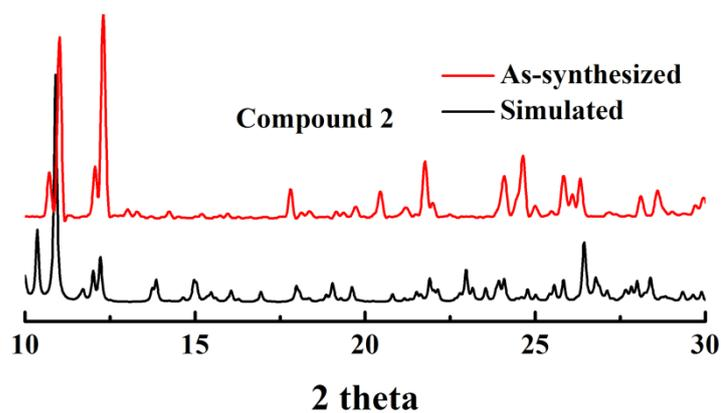
**Fig. S4.** Simulated and experimental XRD spectra of compound 2. Due to the moisture absorption of DMA cations and DMF, partial crystal structures decomposed
