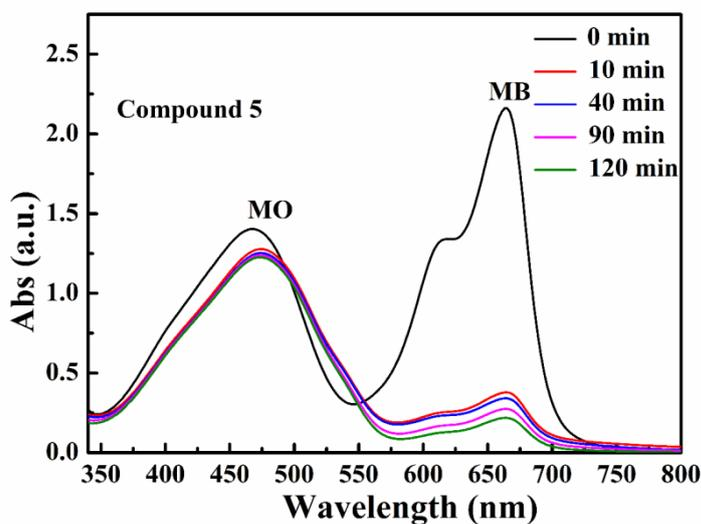
**Fig. S35.** The selective adsorption capability of compound **5** toward the mixed dyes: MO and MB.
