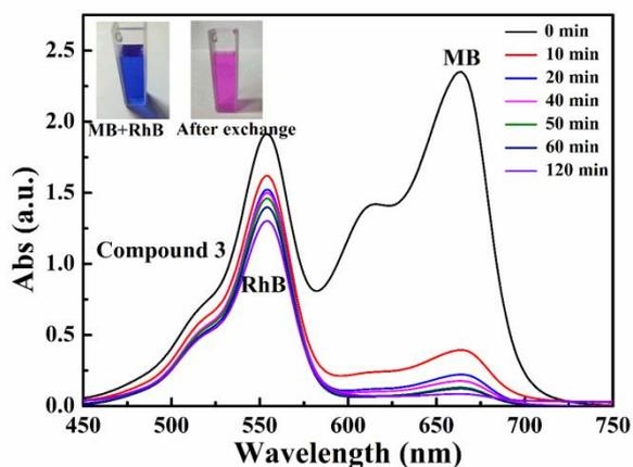
**Fig. S28.** The selective adsorption capability of compound **3** toward the mixed dyes: RhB and MB.
