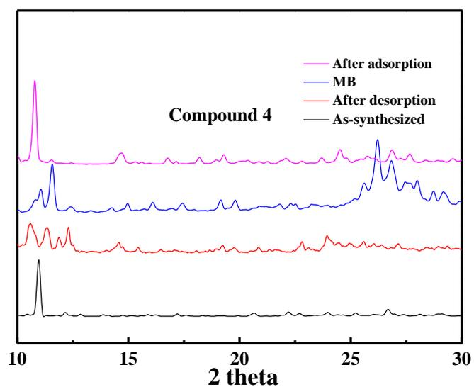
**Fig. S50.** Experimental and After adsorption XRD spectras of compound 4
