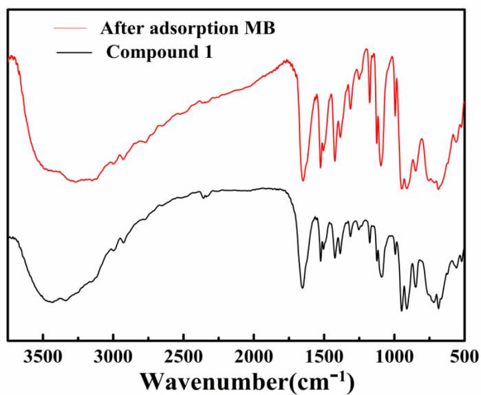
**Fig. S20.**IR spectra of the final recycled powdered solidand compound 1.
