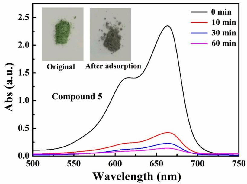
**Fig. S19.**Compound 5 was used to adsorb MB (10 mg/L, 100 mL) aqueous solution
