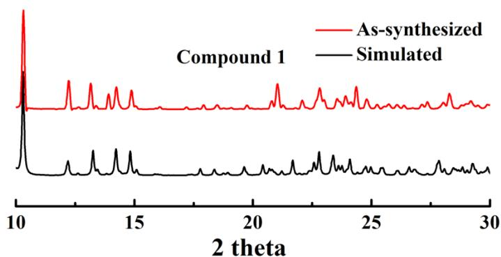
**Fig. S3.** Simulated and experimental XRD spectra of compound 1
