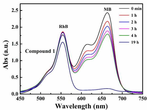
**Fig. S26.** The selective adsorption capability of compound 1 toward the mixed dyes: RhB and MB.
