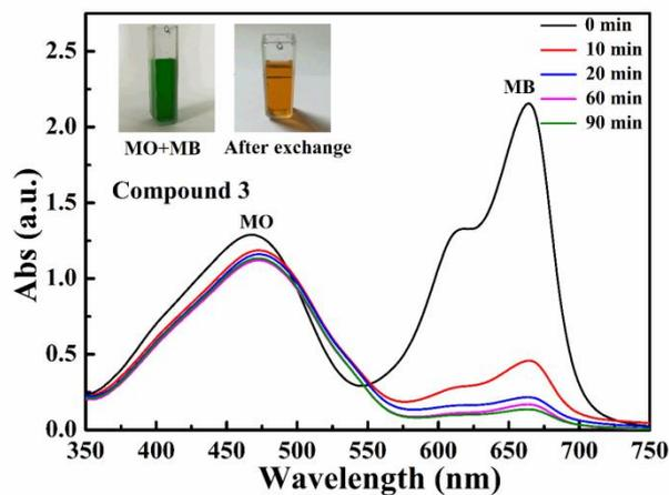
**Fig. S33.** The selective adsorption capability of compound **3** toward the mixed dyes: MO and MB.
