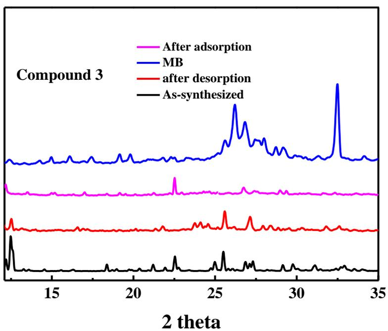
**Fig. S49.** Experimental and after adsorption XRD spectra of compound 3
