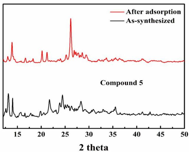
**Fig. S51.** Experimental and after adsorption XRD spectras of compound 5
