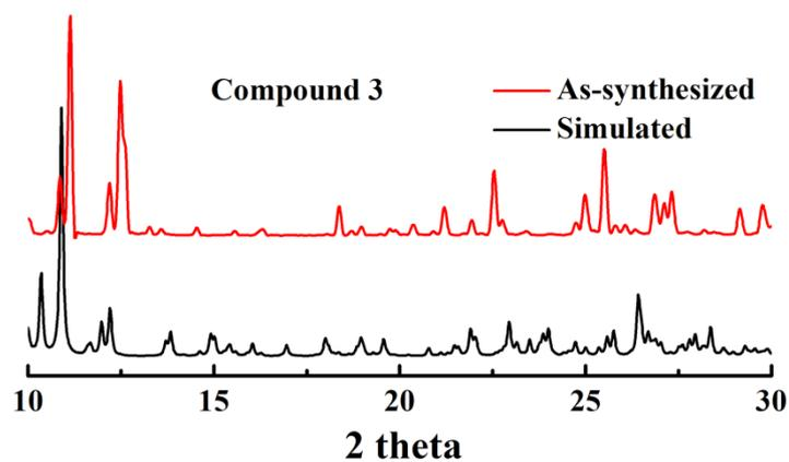
**Fig. S5.** Simulated and experimental XRD spectra of compound 3. Due to the moisture absorption of DMA cations and DMF, partial crystal structures decomposed.
