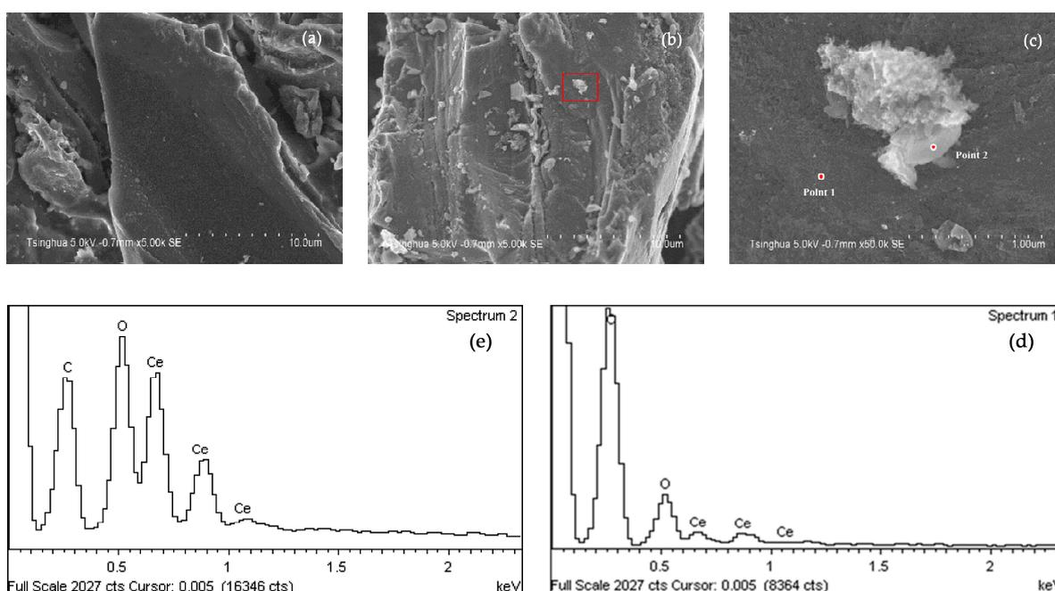
**Figure 1.** SEM and EDS analysis results: (a) SEM of AC-A; (b,c) SEM of Ce/AC; (d) EDC of Point 1; (e) EDS of Point 2.
