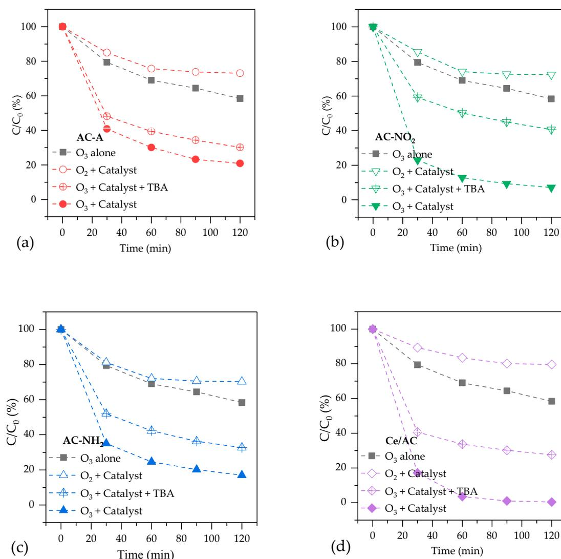
**Figure 2.** The removal of p-CBA by catalytic ozonation with four catalysts: (a) AC-A, (b) AC-NO<sub>2</sub>, (c) AC-NH<sub>2</sub> and (d) Ce/AC.
