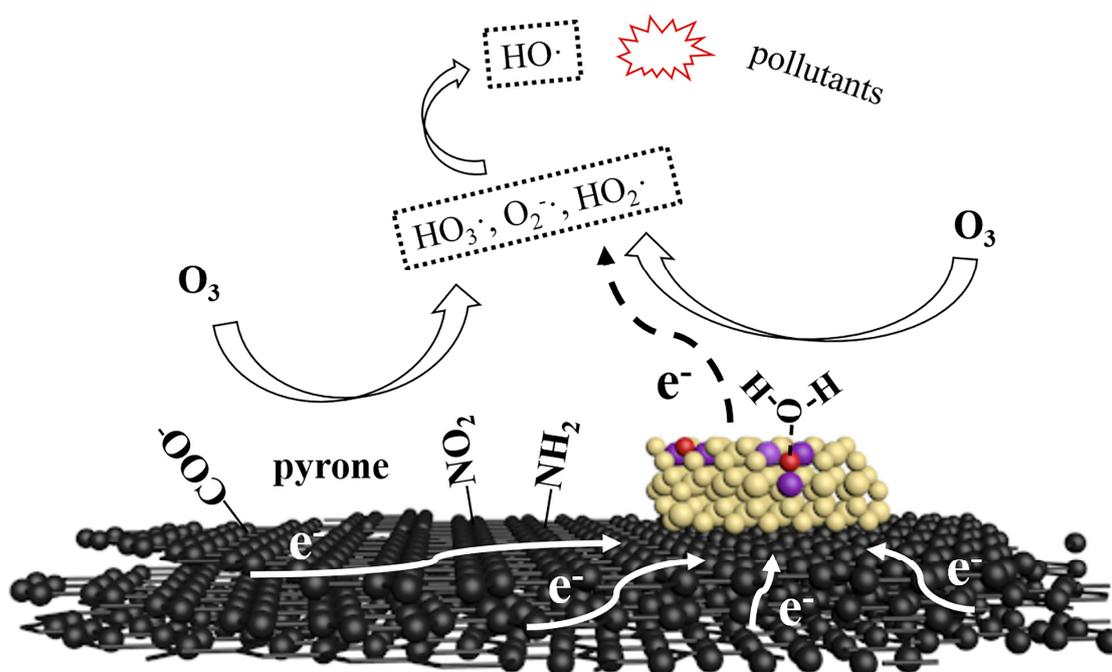
**Figure 4.** A possible mechanism for generation of  $\cdot\text{OH}$  in catalytic ozonation system with Ce/AC. black: graphene; brown: cerium oxide; red: oxygen vacancy; purple:  $\text{Ce}^{3+}$ .
