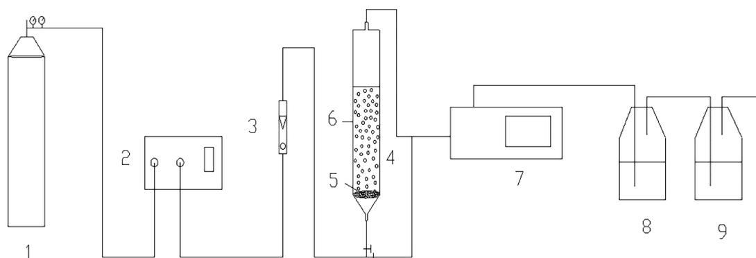
**Figure 5.** Experimental System (1) Oxygen bomb; (2) Ozone generator; (3) Gas flowmeter; (4) Tubular borosilicate glass oxidation reactor; (5) Aeration plate; (6) Sampling port; (7) On-line ozone concentration analyzer; (8 & 9) Absorption bottle.
