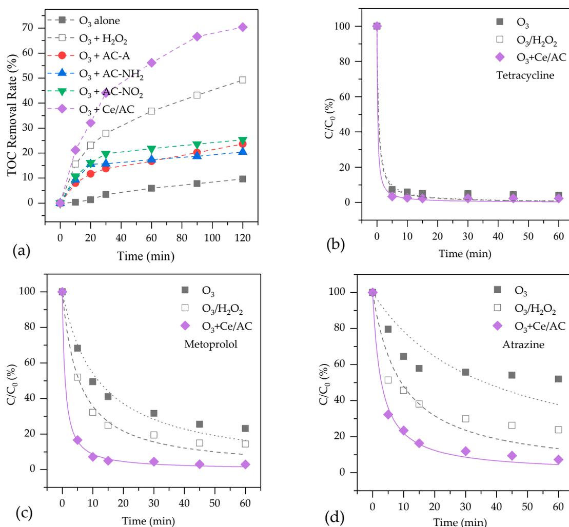
**Figure 3.** The efficiency of organic degradation by  $\text{O}_3$  alone,  $\text{O}_3/\text{H}_2\text{O}_2$  and catalytic ozonation processes in ROC: (a) TOC; (b) Tetracycline; (c) Metoprolol; (d) Atrazine.
