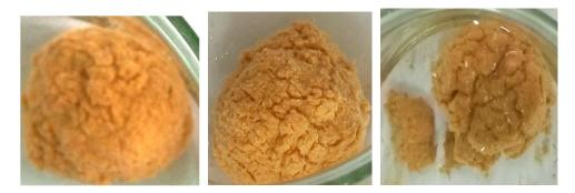
Figure 2. The appearance of mud balls immersed in water for 12 h, 24 h, and 36 h.
