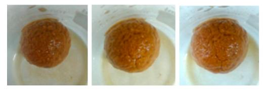
Figure 3. The appearance of mud balls immersed in FCLS-2 for 12 h, 24 h, and 36 h.
