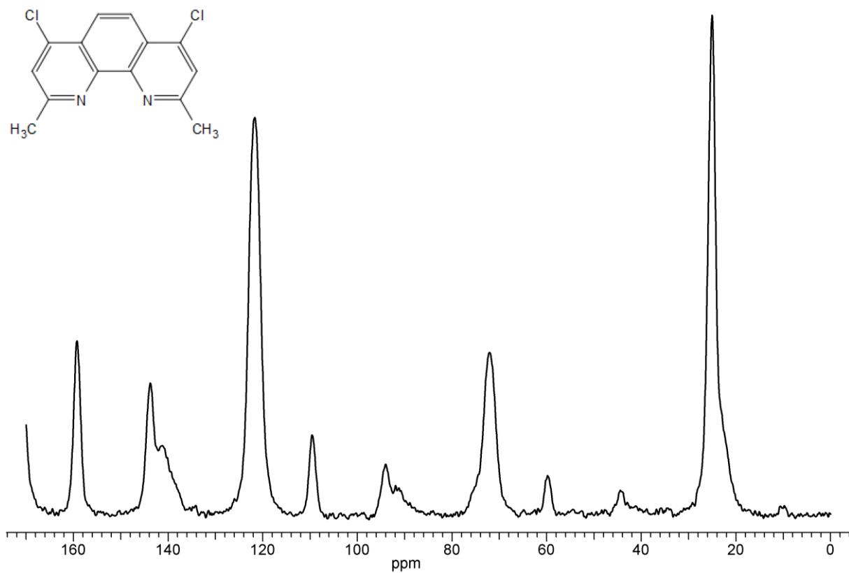
**Fig. S7c.** <sup>13</sup>C CP/MAS NMR spectrum of **4g**.
