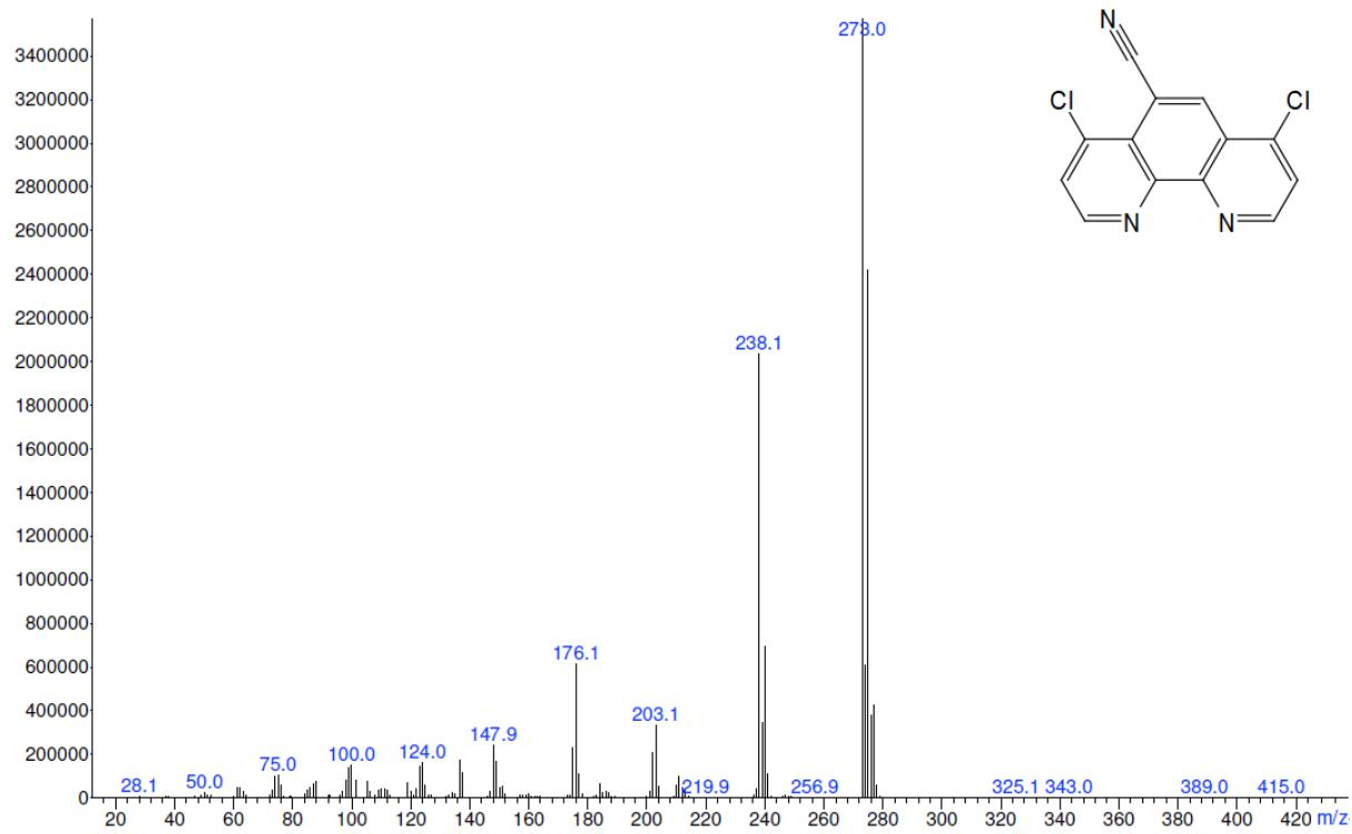
Fig.S5c. MS spectrum of 4e
