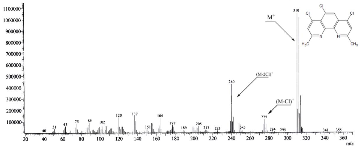
**Fig. S9c.** MS spectrum of **4i**.
