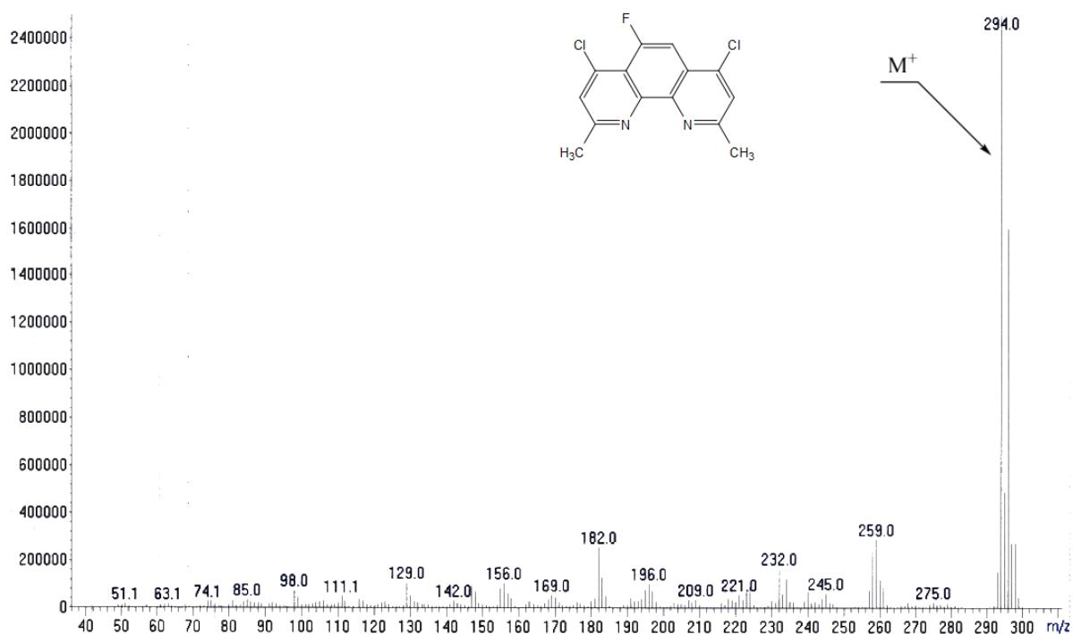
**Fig. S8e.** MS spectrum of **4h**.
