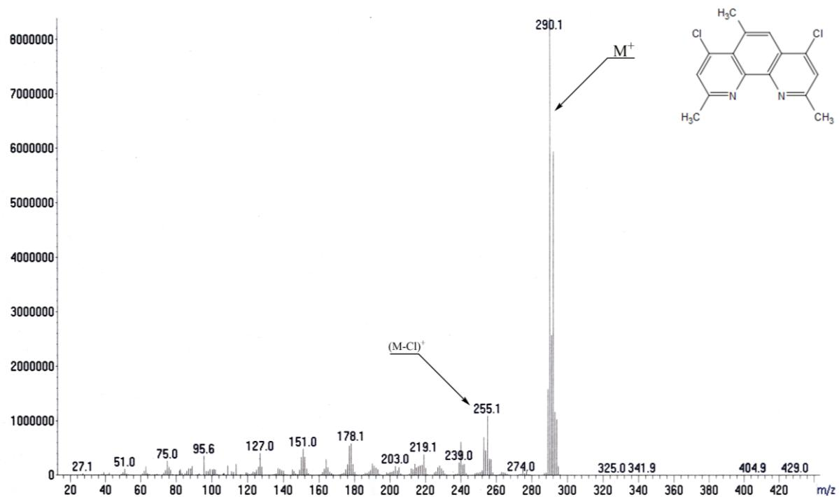
**Fig. S11e.** MS spectrum of **4k**.
