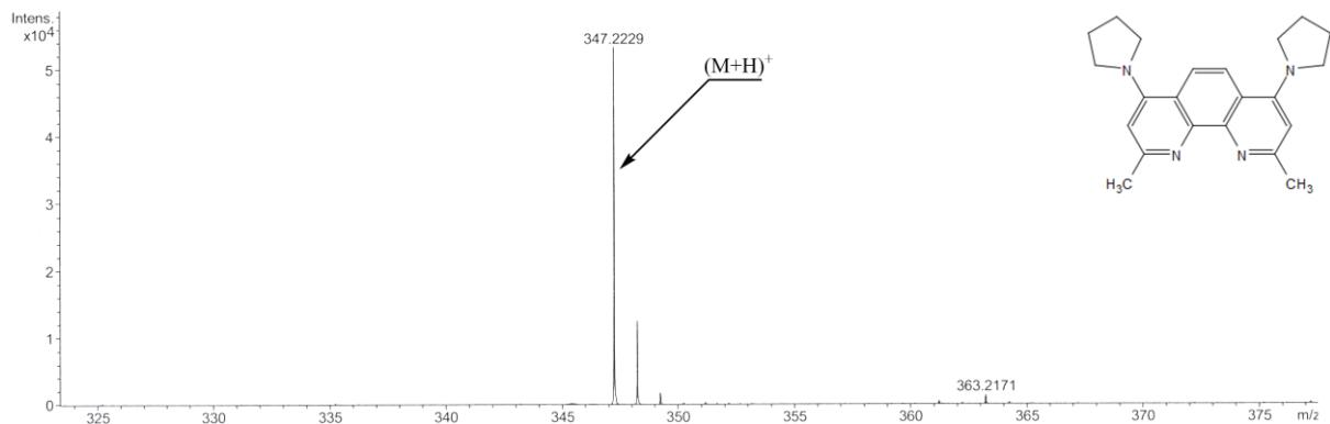
**Fig. S16e.** MS spectrum of **5c**.
