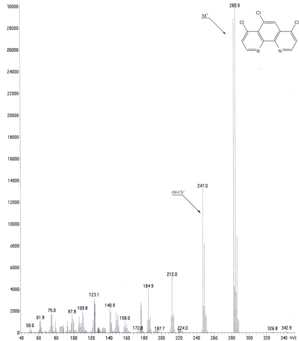
**Fig. S3c.** MS spectrum of **4c**.
