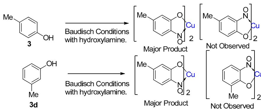
**Scheme 10.** The results of reactions of methyl-substituted phenols show that the favoured product has the methyl group *para* to the nitroso (n.b. given of course the nitroso must also be *ortho* to the phenol).
