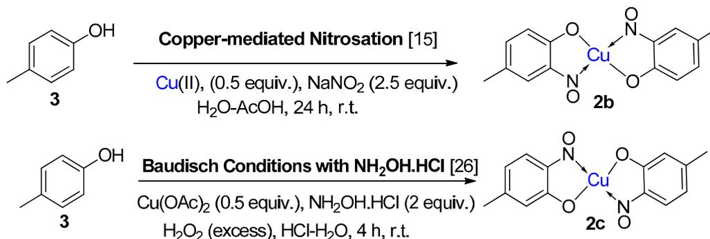
**Scheme 2.** A clear distinction between copper-mediated aromatic nitrosation of phenols and the Baudisch conditions is demonstrated by the reporting of a different major product from the same starting material (3) [15,26].
