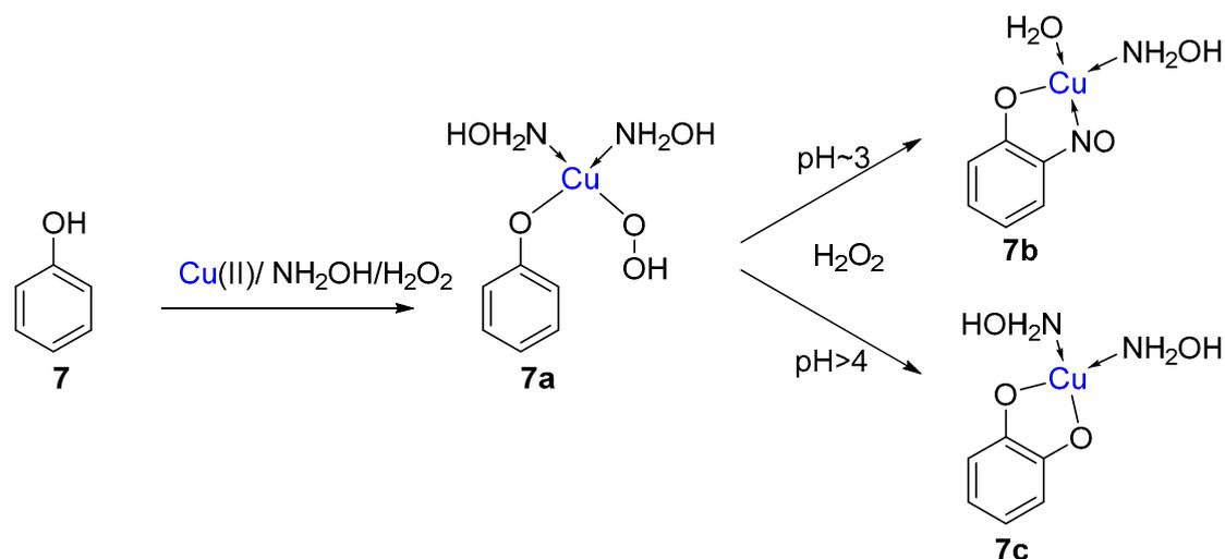
**Scheme 5.** The suggested common intermediate complex (**7a**) between the reactions at different pH. At a  $\text{pH} \sim 3$ , the favoured path leads to the copper 2-nitrosophenol complex (**7b**), while at a  $\text{pH} > 4$  the preferred pathway leads to catechol (**7c**).
