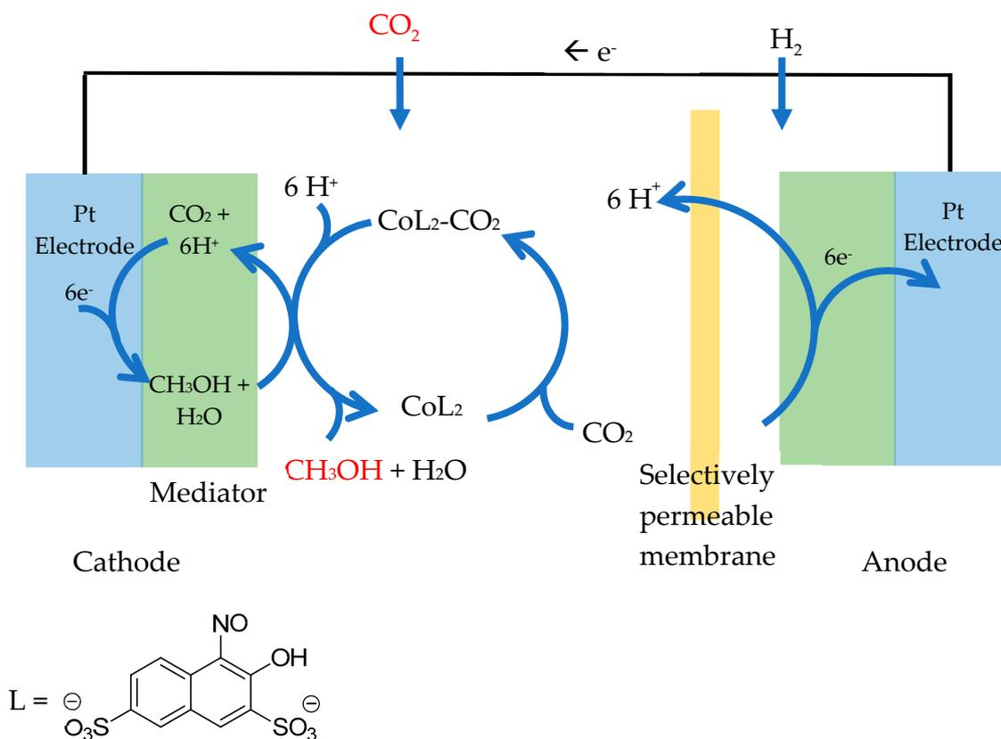
**Figure 11.** An adapted diagram to show the Catalytic reduction of  $\text{CO}_2$  to methanol. Overall equation:  $\text{CO}_2 + 3\text{H}_2 \rightarrow \text{CH}_3\text{OH} + \text{H}_2\text{O}$  [72].
