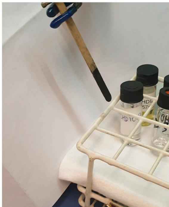
**Figure 1.** Coated graphene oxide/polyethylene glycol (GO/PEG)-Stick.
