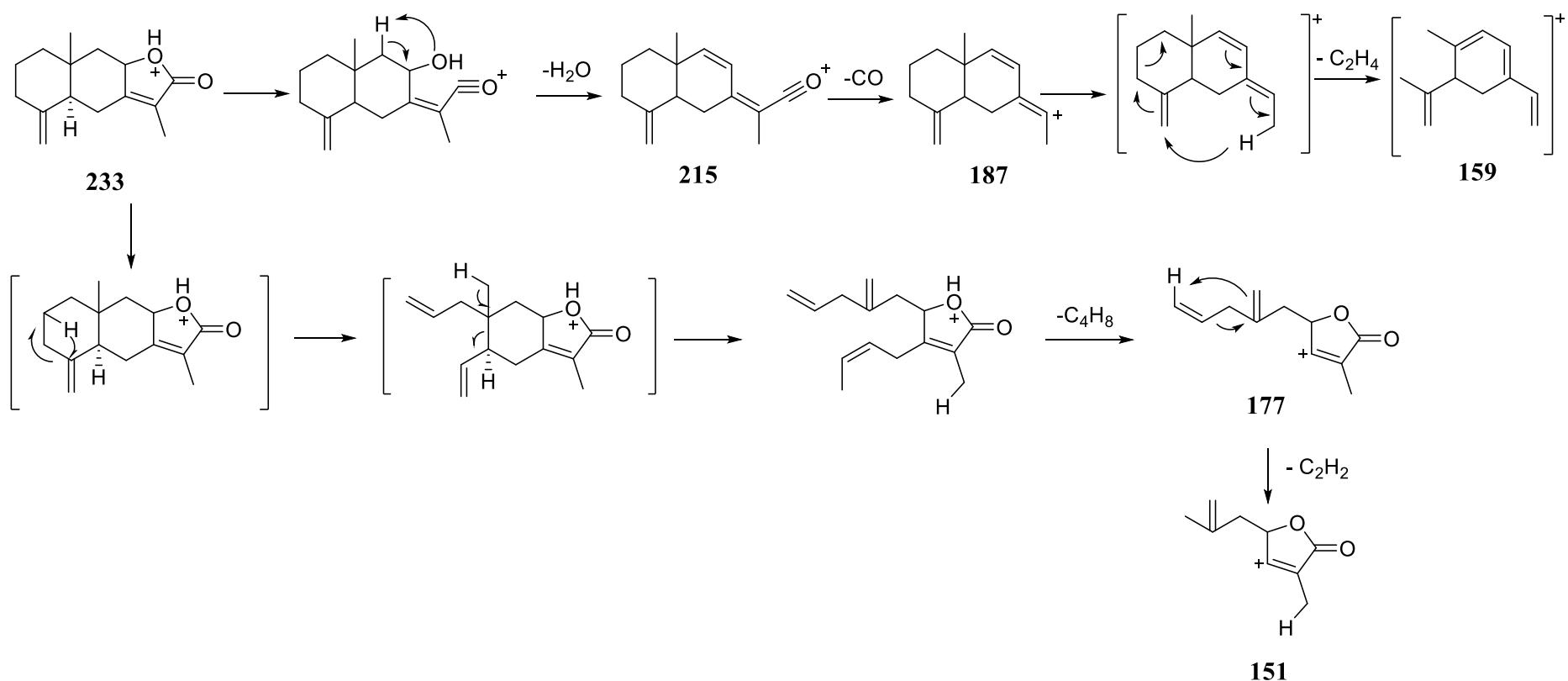
The fragmentation pathway of atracylenolide I were analyzed using a high-resolution linear ion trap Orbitrap mass spectrometer
