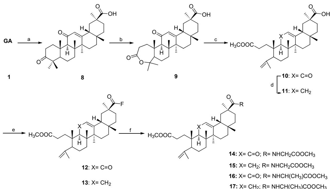
**Scheme 2.** Reagents and conditions: (a) Jones reagent, acetone, 0 °C; (b) *m*-CPBA, CH<sub>2</sub>Cl<sub>2</sub>, r.t.; (c) MeOH, *p*-TSA, CH<sub>2</sub>Cl<sub>2</sub>, r.t.; (d) zinc dust, conc. HCl, dioxane, r.t.; (e) Deoxo-Fluor®, CH<sub>2</sub>Cl<sub>2</sub>, r.t.; (f) glycine methyl ester hydrochloride or L-alanine methyl ester hydrochloride, Et<sub>3</sub>N, CH<sub>2</sub>Cl<sub>2</sub>, r.t.
