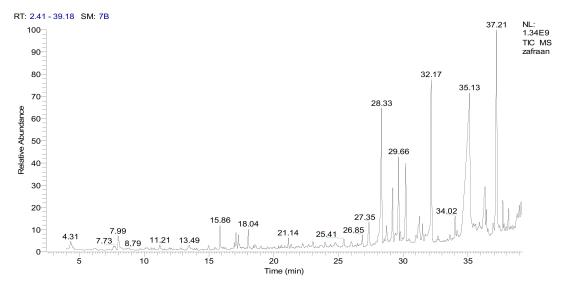
**Figure 3.** The TIC chromatogram of CSME using GC-MS. RT- Retention Time; SM- Signal in Method; NL-Noise Level.
