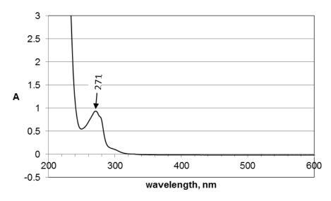
**Figure S3.** UV-visible absorption spectrum of paraffin oil recorded by a Shimadzu UV-2450 spectrophotometer.
