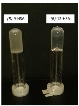
**Figure S2.** 1 % w/w gel samples in paraffin oil prepared by microwave irradiation. In each sample there is a small magnetic stirrer bar.
