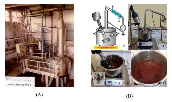
**Figure 3.** (**A**) Industrial turbo-Clevenger; (**B**) laboratory turbo-Clevenger: (**a**) schematic, (**b**) bench apparatus, (**c**) cinnamon experiment before extraction with mixer detail (insert), (**d**) cinnamon experiment after extraction.
