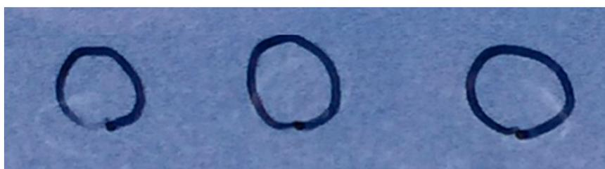
**Figure 6.** Photograph of three 10  $\mu\text{L}$  drops of 50 ng/mL fentanyl dried on part of a glass slide. This concentration corresponds to 500 pg. The samples, deposited on the opposite side of the  $\sim 5\text{ mm}$  diameter black marked rings, migrated during evaporation, forming nearly invisible white rings.
