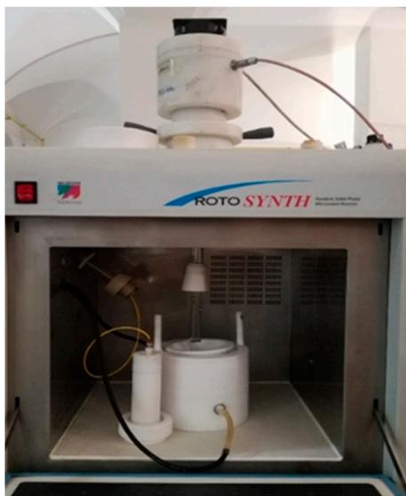
**Figure 8.** Combined MW/US device.
