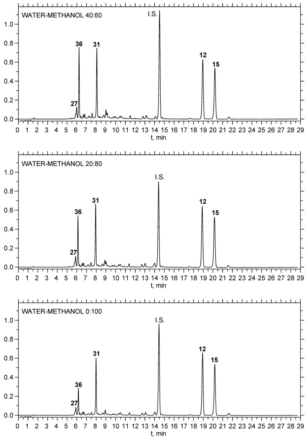
**Figure S5.** mcHPLC-UV chromatograms of *P. sibiricus* herb extracts prepared with various solvents. Compounds numbered as **11** – khellactone 4'-*O*-angeloyl ester (d-laserpitin), **15** – khellactone 3'-*O*-isovaleroyl-4'-*O*-acetyl ester (dihydrosamidin), **27** – umbelliferone-7-*O*-(6'-apiosyl)-glucoside (6'-apiosylskimmin), **31** – khellactone-3'-*O*-glucoside (praeroside II), **36** – 5-*O*-caffeoylequinic acid. I.S. – internal standard (pimpinellin).
