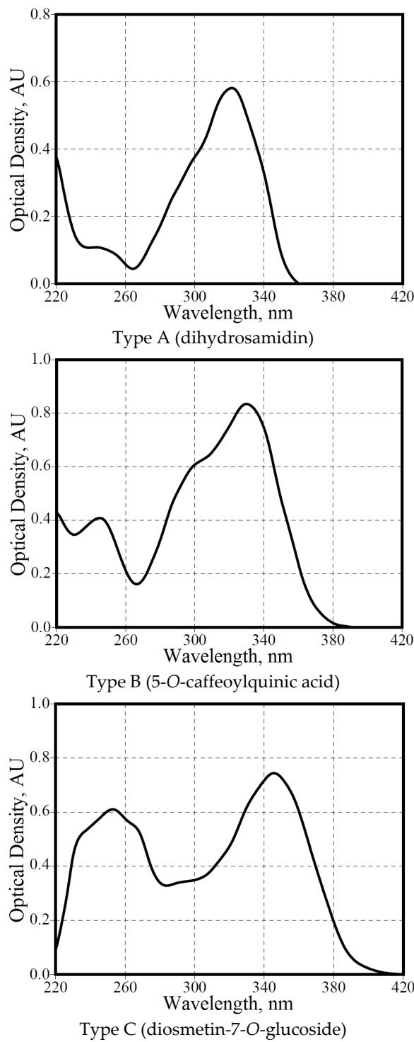
**Figure S3.** Types of UV spectral patterns.
