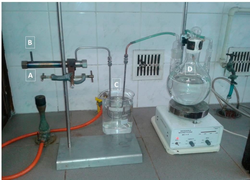
**Figure 2.** The instrumentation designed for laboratory tests of the method of processing zinc-ferric waste materials: furnace (A) for roasting and carbothermic decomposition of zinc ferrite, air access (B), heat exchanger (C), SO<sub>2</sub> water collector (D)—production of leaching agent.
