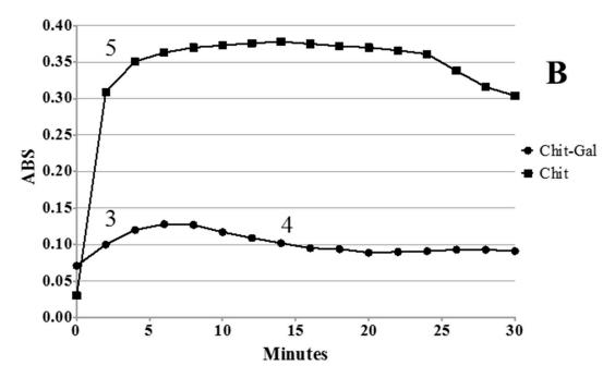
**Figure 3.** Formation profile of CaOx crystals. **A.** Formation profile in control condition and in the presence of chit-gal. **B.** Formation profile in the presence of chit-gal and Chit. 1, 3, and 5 indicate nucleation/growth phases. 2 and 4 indicate aggregation phase.
