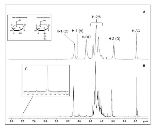
**Figure 2.** NMR spectra for Chit (**A**) and Chit-Gal (**B**). The identified signals correspond to the typical signs of Chit, present in both samples. H-AC corresponds to the hydrogens of the methyl group of N-acetylglucosamine; D and A correspond to deacetylated and acetylated unities, respectively. H-OD indicates hydrogens of deuterium oxide. Highlighted is the signal at 7.49 ppm (**C**), present only in the Chit-Gal spectrum and corresponds to the hydrogen from the aromatic ring.
