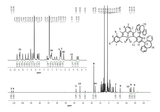
**Figure S4** <sup>1</sup>H NMR spectrum of **Co4** in CD<sub>2</sub>Cl<sub>2</sub> at room temperature.
