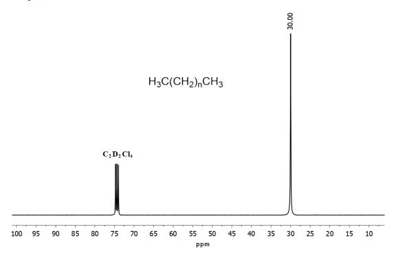
**Figure S12** The <sup>13</sup>C NMR spectrum of the polyethylene obtained with **Co1**/MMAO (Table 5, entry 10).
