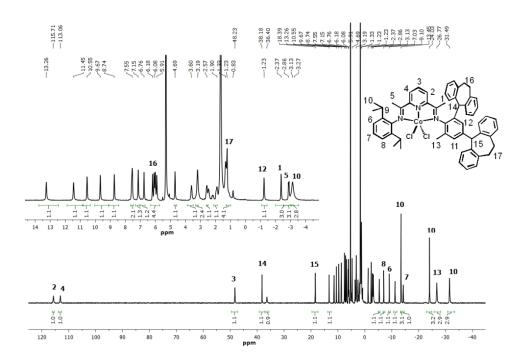
Figure S3 <sup>1</sup>H NMR spectrum of Co3 in CD<sub>2</sub>Cl<sub>2</sub> at room temperature.
