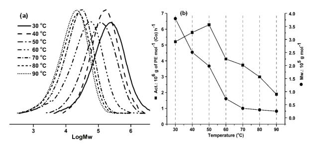
**Figure S6** GPC curves of the obtained polyethylene (a); activity and  $M_w$  as a function of reaction temperature (b) for the **Co1**/MMAO system (Table 5, entries 1-7).
