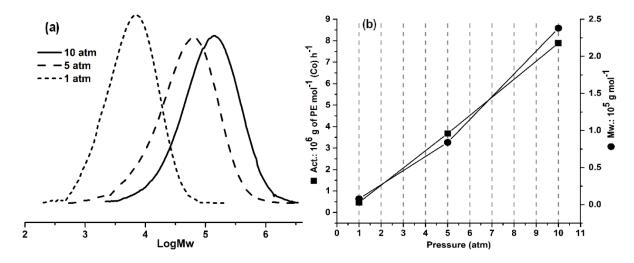
**Figure S10** GPC curves of the obtained polyethylene (**a**); activity and  $M_w$  as a function of ethylene pressure (**b**) at the optimized reaction conditions for the **Co1**/MMAO system (Table 5, entries 10, 18 and 19).
