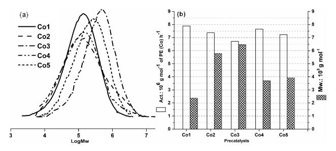
Figure S9 GPC curves of the obtained polyethylene (a); activity and  $M_w$  for different precatalysts (b) at the optimized reaction conditions with MMAO as cocatalyst (Table 6, entries 1-5).
