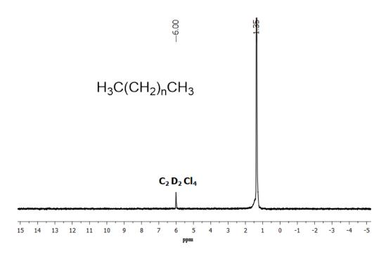
**Figure S11** The <sup>1</sup>H NMR spectrum of the polyethylene obtained with **Co1**/MMAO (Table 5, entry 10).
