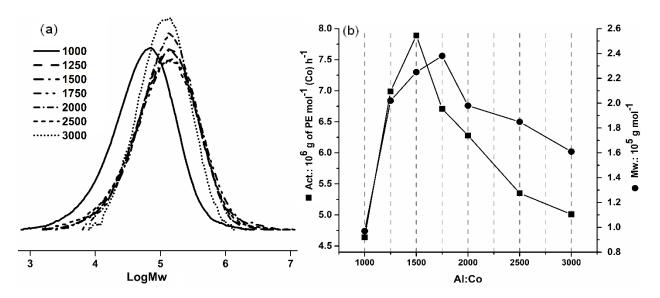
**Figure S7** GPC curves of the obtained polyethylene (a); activity and  $M_w$  as a function of Al/Co ratio (b) for the Co1/MMAO system (Table 5, entries 3 and 8 – 13).
