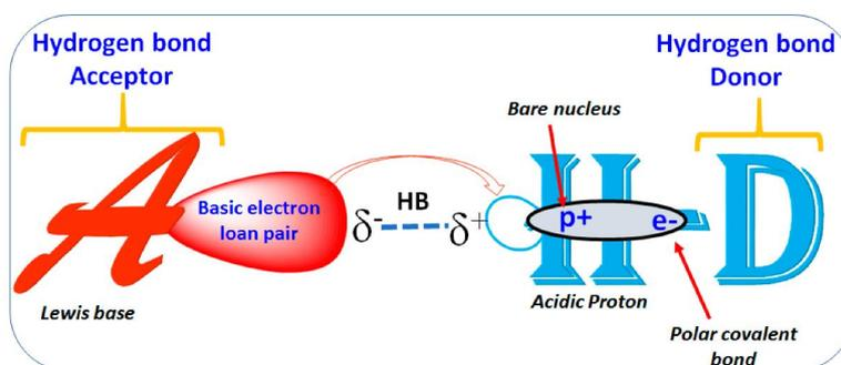
**Figure 2.** The pictorial illustration of hydrogen bond interaction, where HB acceptor/donor can be an F, O, N, or S atom in the molecule. Electron polarization and exposure of a positive proton on either side are shown schematically.
