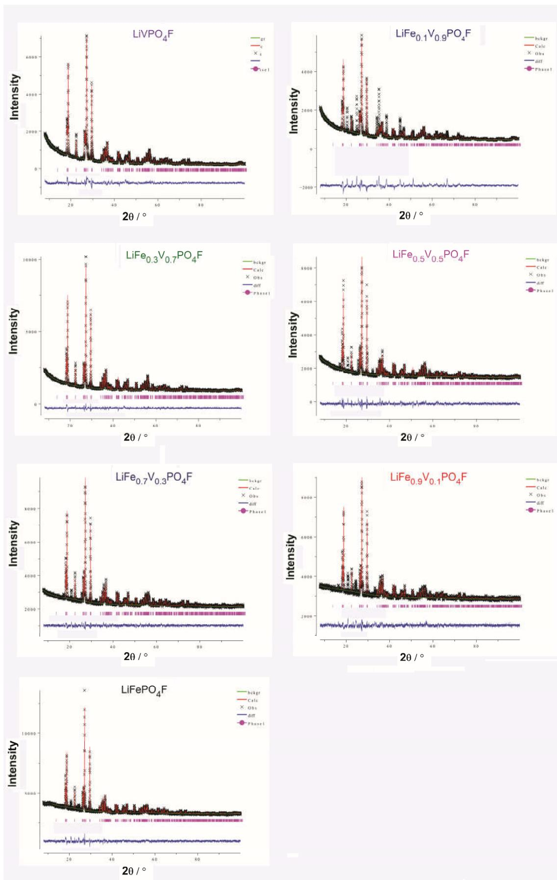
**Figure S1.** The final observed, calculated and difference profiles of the tavorite-structured  $\text{LiFePO}_4\text{F}$  (a),  $\text{LiFe}_{0.9}\text{V}_{0.1}\text{PO}_4\text{F}$  (b),  $\text{LiFe}_{0.7}\text{V}_{0.3}\text{PO}_4\text{F}$  (c),  $\text{LiFe}_{0.5}\text{V}_{0.5}\text{PO}_4\text{F}$  (d),  $\text{LiFe}_{0.3}\text{V}_{0.7}\text{PO}_4\text{F}$  (e),  $\text{LiFe}_{0.1}\text{V}_{0.9}\text{PO}_4\text{F}$  (f) and  $\text{LiVPO}_4\text{F}$  (g) *via* Rietveld refinements.
