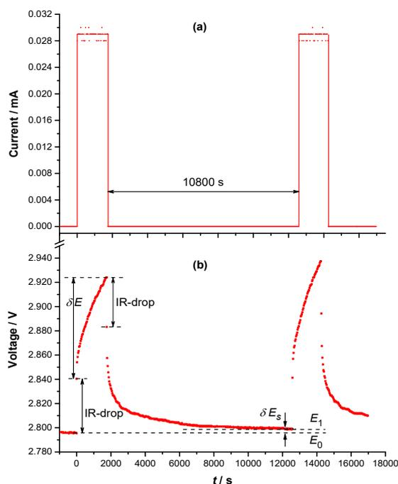
**Figure S3.** Scheme for a GITT measurement. (a) the constant current pulse; (b) potential response.
