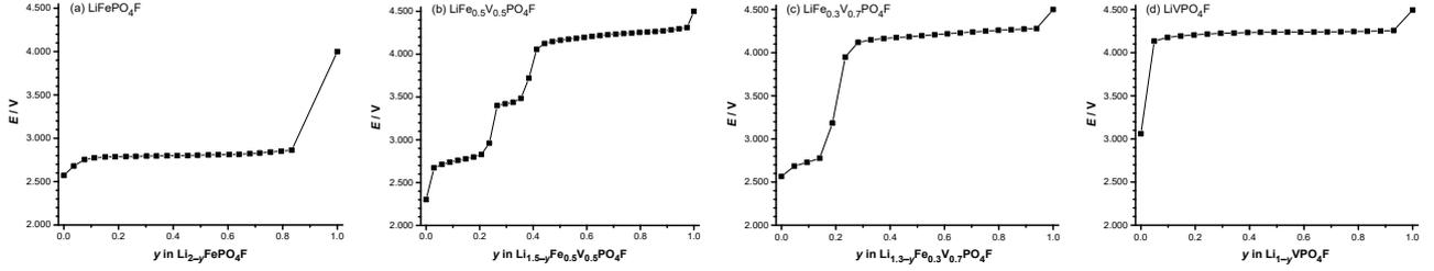
**Figure S5.** Curves of the quasi-equilibrium OCVs as a function of  $\text{Li}^+$ -extraction content  $y$  by GITT in  $\text{Li}_{1-y}\text{Fe}_{1-x}^{\text{III}}\text{V}_x^{\text{III}}\text{PO}_4\text{F}$ , *i.e.*  $\text{Li}_{2-x-y}\text{Fe}_{1-x}^{\text{II}}\text{V}_x^{\text{III}}\text{PO}_4\text{F}$  with  $x = 0$  (a),  $x = 0.5$  (b),  $x = 0.7$  (c) and  $x = 1$  (d).
