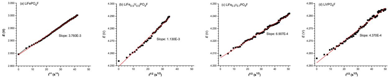
**Figure S7.** Plots of the slope of initial transient voltage change as a function of square root of time ( $\delta E / \delta t^{1/2}$ , within a single charging current pulse duration) and the fitted lines in  $\text{Li}_{1-y}\text{Fe}_{1-x}^{\text{III}}\text{V}_x^{\text{III}}\text{PO}_4\text{F}$ , *i.e.*  $\text{Li}_{2-x-y}\text{Fe}_{1-x}^{\text{II}}\text{V}_x^{\text{III}}\text{PO}_4\text{F}$  with  $x = 0$  (a),  $x = 0.5$  (b),  $x = 0.7$  (c) and  $x = 1$  (d).
