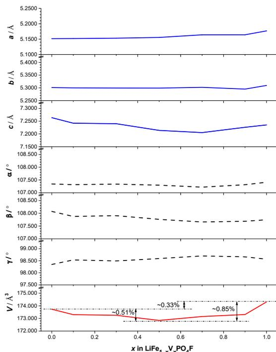
**Figure S2.** Variations of lattice parameters ( $a$ ,  $b$ ,  $c$ ,  $\alpha$ ,  $\beta$  &  $\gamma$ ) and unit cell volumes ( $V$ ) of  $\text{LiFe}_{1-x}\text{V}_x\text{PO}_4\text{F}$  ( $0 \leq x \leq 1$ ) solid solutions.
