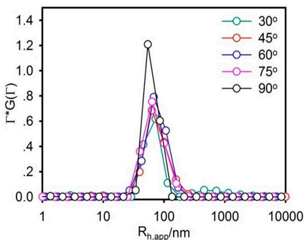
**Figure 1.** Size distribution of deoxyschizandrin and its liposome (DS-lipo).  $q\varrho/l = 1.0$ . Temperature = 37 °C.
