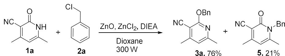
**Scheme 3.** Microwave-assisted benzylation of **1a** and **2a**.
