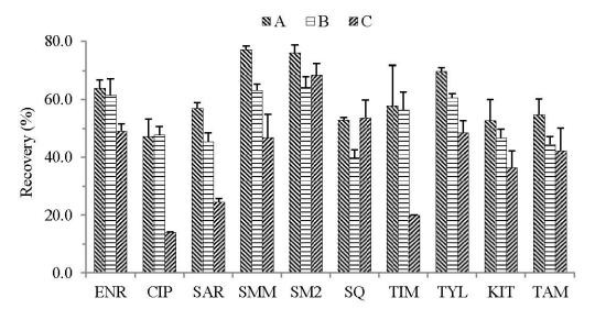
**Figure 1.** Influence of different extraction solvents on the recoveries of compounds in the chicken muscle sample at the spiked 50  $\mu$ g kg<sup>-1</sup> (*n* = 5), (A) Acetonitrile, (B) Methanol, (C) Ethyl acetate.
