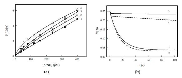
**Figure 2.** (a) Rates of oxidation of  $100~\mu M$  NADPH by nitrosobenzene in the absence (1) and presence of NfsA (2–4). Enzyme concentration, 10~n M (2), 20~n M (3), and 40~n M (3); (b) Kinetics of oxidation of  $100~\mu M$  NADPH by  $400~\mu M$  nitrosobenzene in the absence (1,3) and presence (2,4) of 40~n M NfsA. Ascorbate (final concentration, 2~m M) was added into a syringe containing NADPH (3,4).
