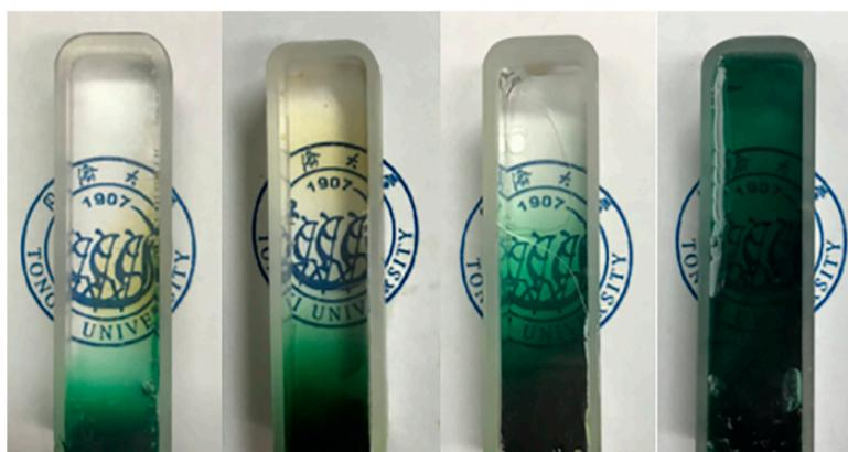
Figure 7. The diffusion process of  $\text{Fe}^{2+}$  into the gel before supercritical drying with the mold of cuvette.
